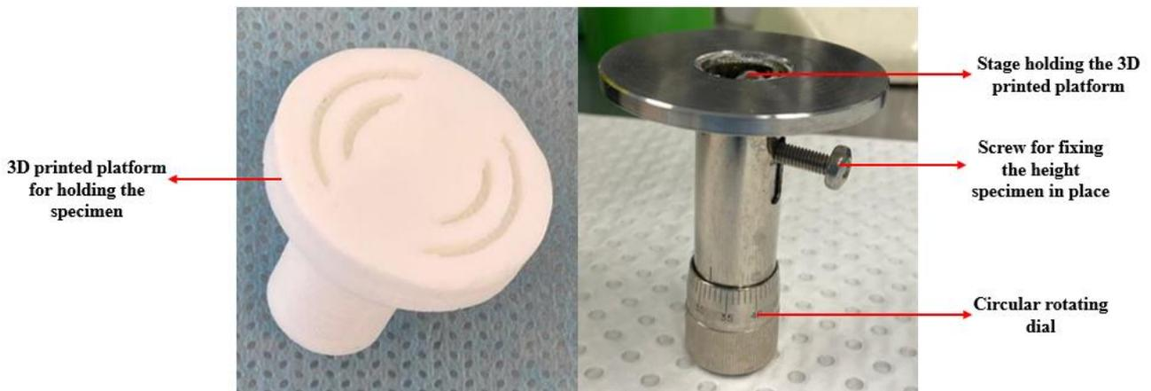
Figure 2: Parts of hand-held microtome
