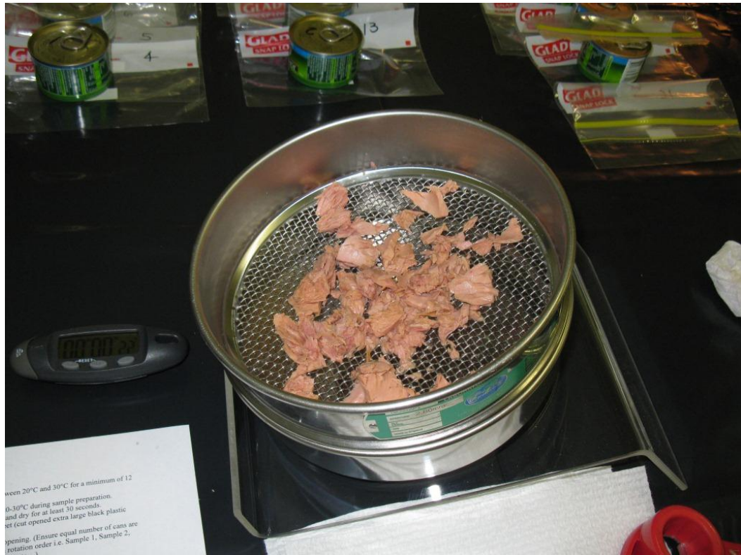
Figure 5.1 Illustration of the draining process for canned fish
