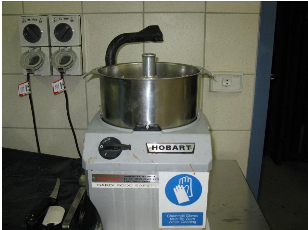
Figure 5.2 Equipment used to homogenise samples
