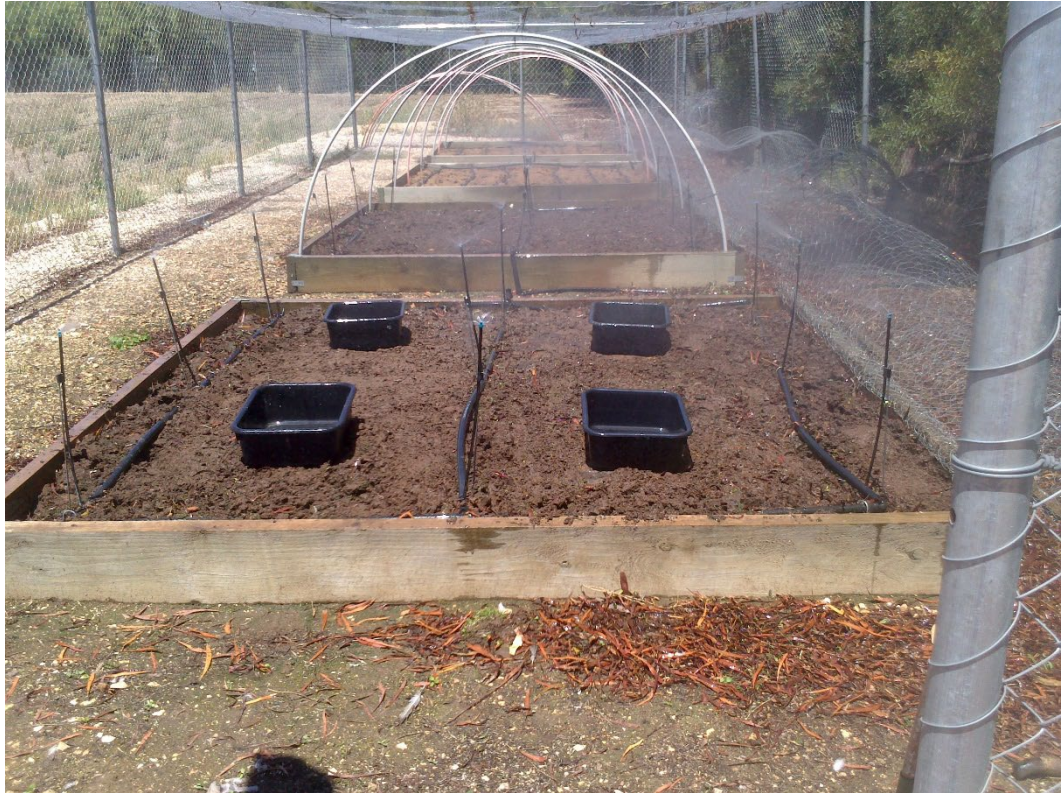
Plate 2. 2 Automated irrigation control unit (a) and Irrigation calibration by using the known area trays (b), Mount Barker, SA, 2016
