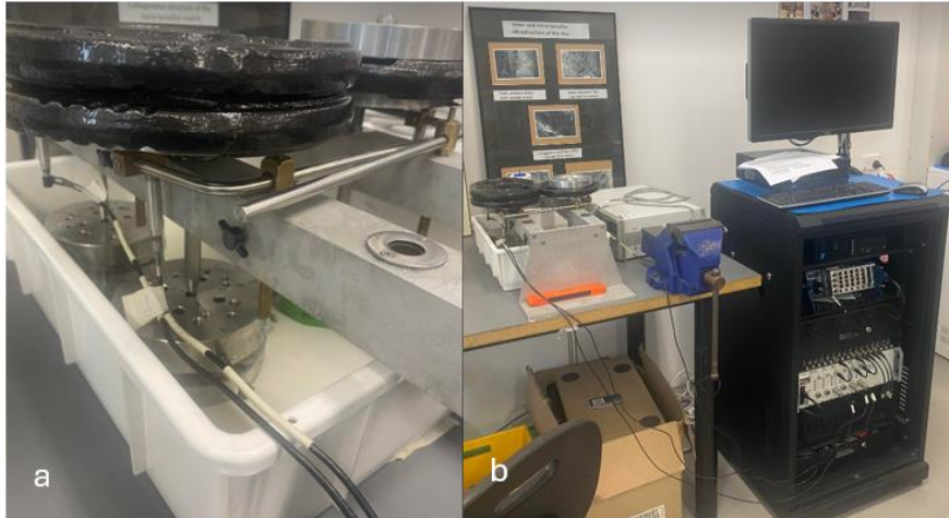
Figure 5a:Specimen hydration under preload, b: hydration set up
