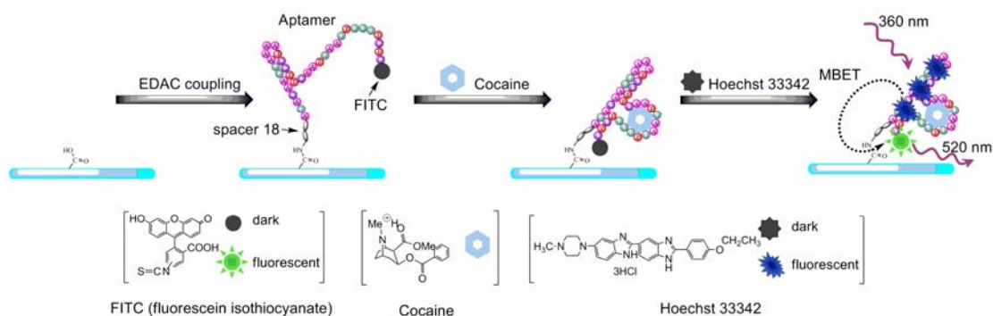
Scheme 6-1. Schematic illustration of MBET aptamer sensors for cocaine detection on a MP2 surface.
