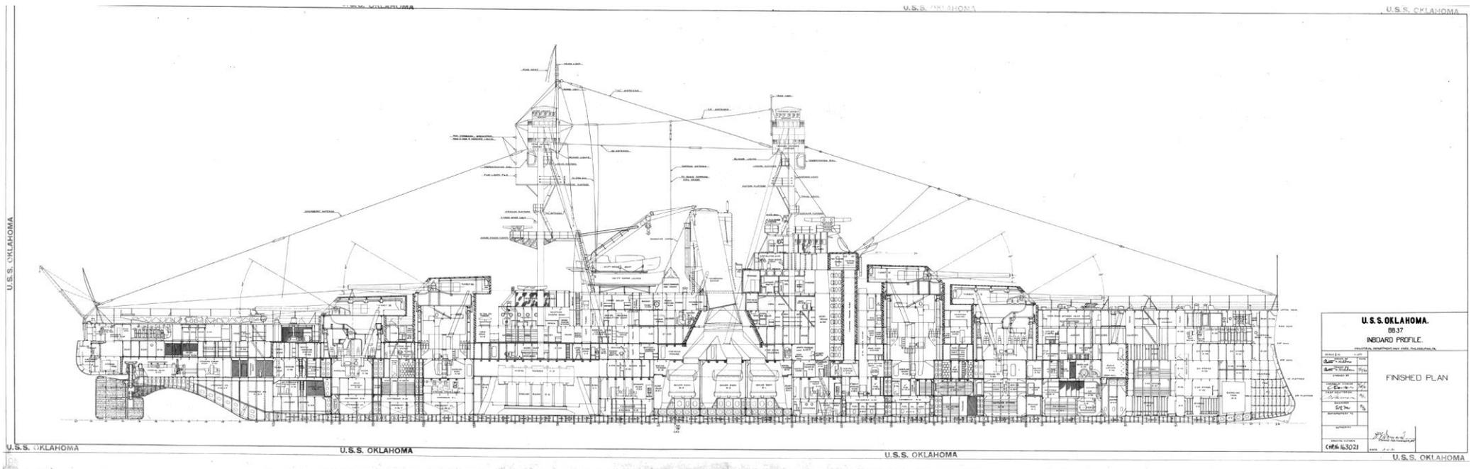
**Figure 5.1.** The inboard profile of the USS *Oklahoma* [13]. The USS *Oklahoma*, also known as BB-37, was a *Nevada*-class battleship that ran fully on liquid fuel. Much of the very bottom of the ship was dedicated to storage of fuel oil.
