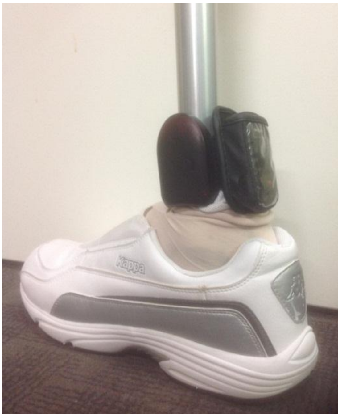
Figure 6.1: The SAM and GPS devices attached to a prosthesis for data collection.
