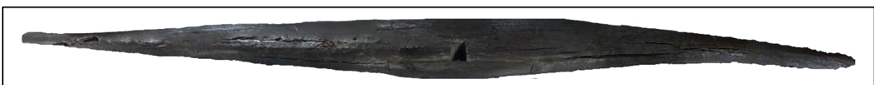
Figure 3.6: A top-down orthophotograph of the Gokstad anchor stock, showing its cylindrical, tapering design (photogrammetry by Author, with the permission of the Viking Ship Museum, Oslo).
