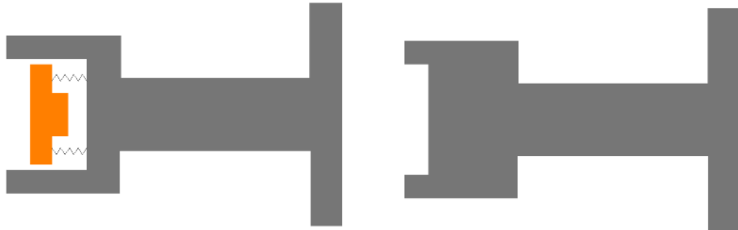
Figure19 : Adjusting spool (spindle) with plate or placoid (orange body) in the left and modified adjusting spool in the right.
