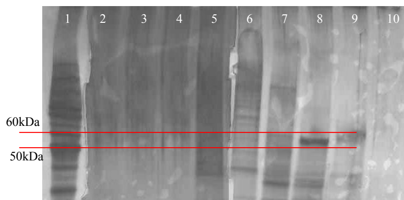
Figure 17. Silver stained SDS-PAGE of fractions from GF-HPLC. Lane Descriptions: 1 – BenchMark Marker (2 \mu L, Invitrogen); 2 – fraction 1; 3 – fraction 3; 4 – fraction 5; 5 – fraction 7; 6 – fraction 9; 7 – fraction 11; 8 – fraction 13; 9 – fraction 15; 10 – fraction 19. 10 \mu L of sample was loaded per well.
