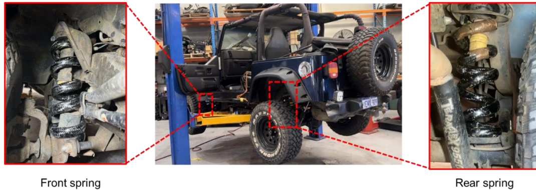
Fig. 8.8 The installation experiment of optimal front and rear TBCHSs.
