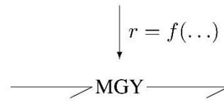
Figure 17 Graphical representation of Modulated gyarator
