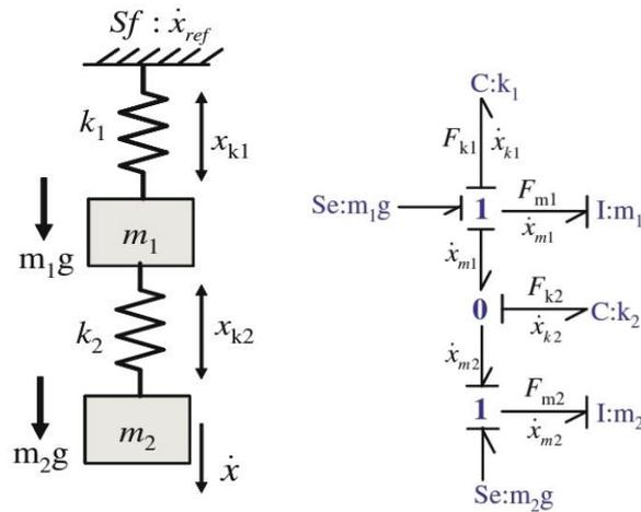
Figure 28 Mechanical double oscillator and corresponding bondgraph
