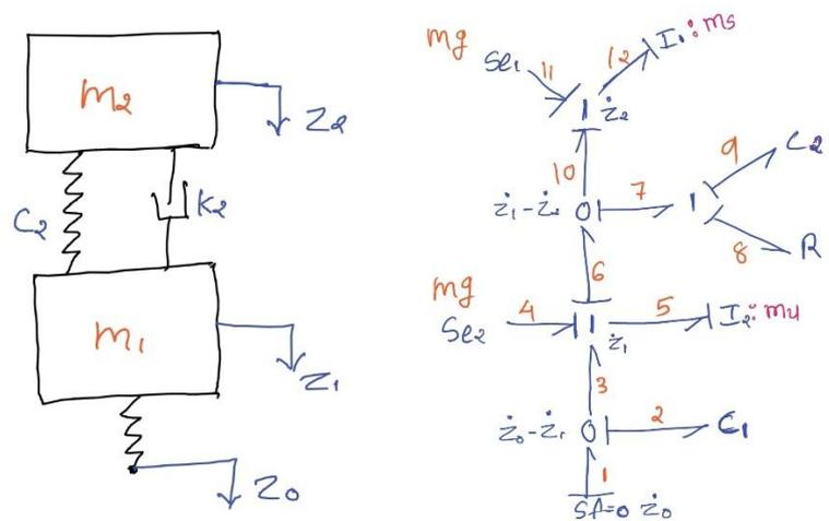
Figure 29 Bond graph model of two degrees of freedom suspension system
