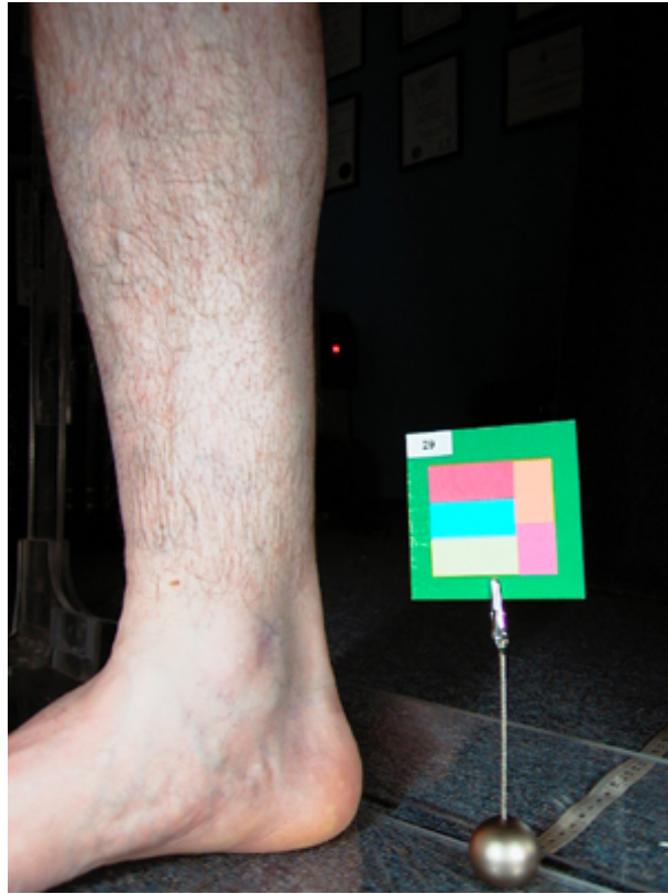
Figure 31. Method used for testing the effect of illumination and different distances from the colour reference
