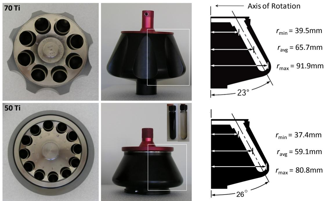
**Figure 2.3:** Rotors used for ultracentrifugation of CNT solutions of different volume and their radii of rotation; Type 70 Ti (top) employed for 25mL volumes and Type 50 Ti (bottom) used for 10mL volumes. Inset: Centrifuge tube with CNT dispersion both prior to centrifugation (black liquid) and after spinning at 43000rpm for 1hr in the 50 Ti rotor showing sedimentation at the tube base and along the wall.
