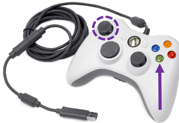
Figure 5-5 – The Microsoft Xbox 360 wired controller, on which the controller hardware needed to be based. The left thumb-stick is highlighted (dashed purple circle), as is the green ‘A’ button (purple arrow). (Source: https://commons.wikimedia.org/wiki/File:Xbox-360-Wired-Controller.jpg )
