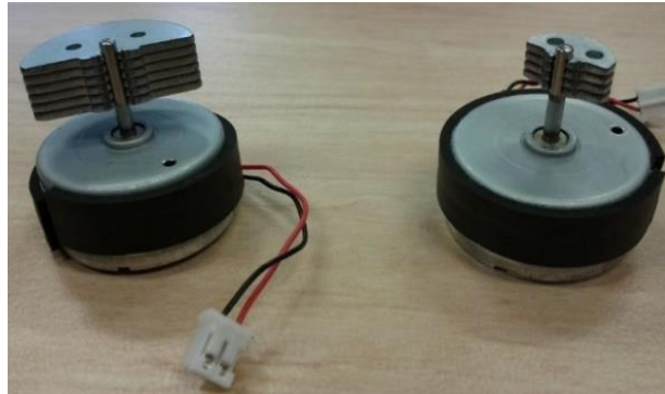
Figure 5-6 – The large (left) and small (right) counterweighted vibration motors taken from a commercial Microsoft Xbox 360 controller
