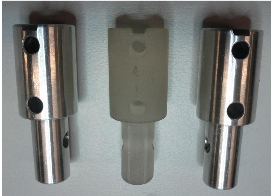
Figure 6-12 – The new machined aluminium pins (left and right), either side of a 3D printed pin (middle)
