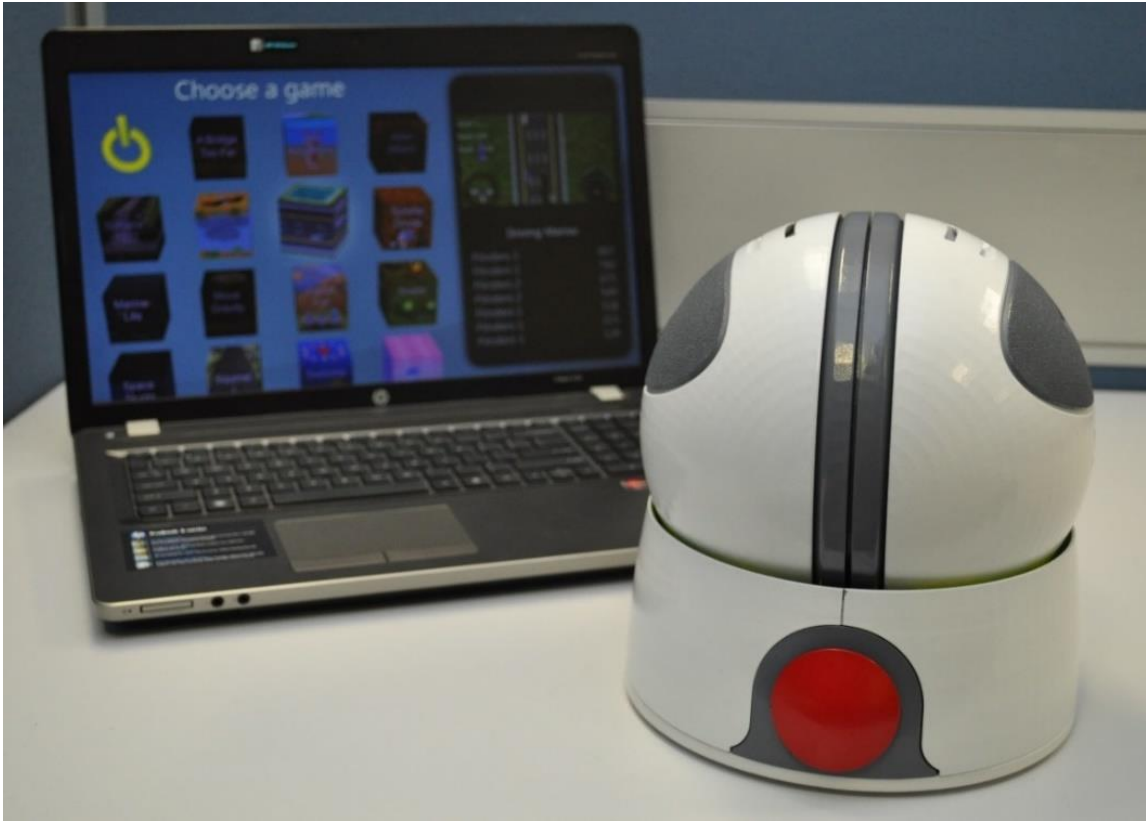
Figure 5-17 – The final OrbIT Gaming System (OGS), showing the Stage 3 ‘Orby’ controller in the foreground and the laptop that runs the software and games in the background
