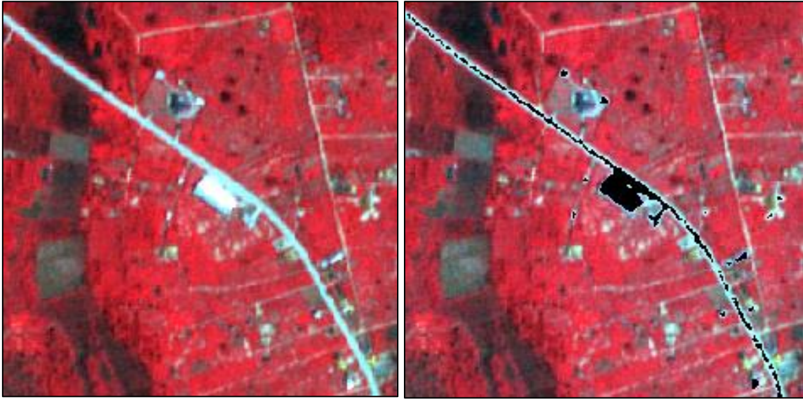
Figure 4.3: The effects of cloud and shadow removal on other ground surface features, PlanetScope displayed in true-colour composite
