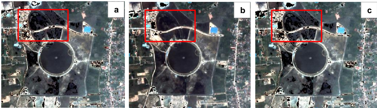
Figure 3.6: Cloud masking image from unsupervised classification (a), a single band threshold (b) and the combination of classification and a single band threshold methods (c) displayed in true-colour composite
