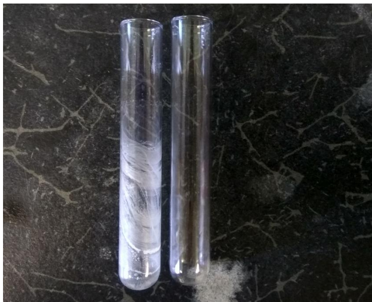
Figure 5-21: Comparison of ammonia in methanol extract evaporation with (left) and without (right) the addition of hydrochloric acid.
