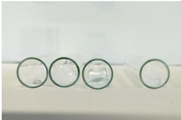
Appendix Figure 17: Side view of droplet with images of in order from left to right each tube is: 10 \mu L milli Q water on silanised glass tube, 10 \mu L milli Q water on unmodified glass tube, 100 \mu L milli Q water on silanised glass tube and 100 \mu L milli Q water on unmodified glass tube.
