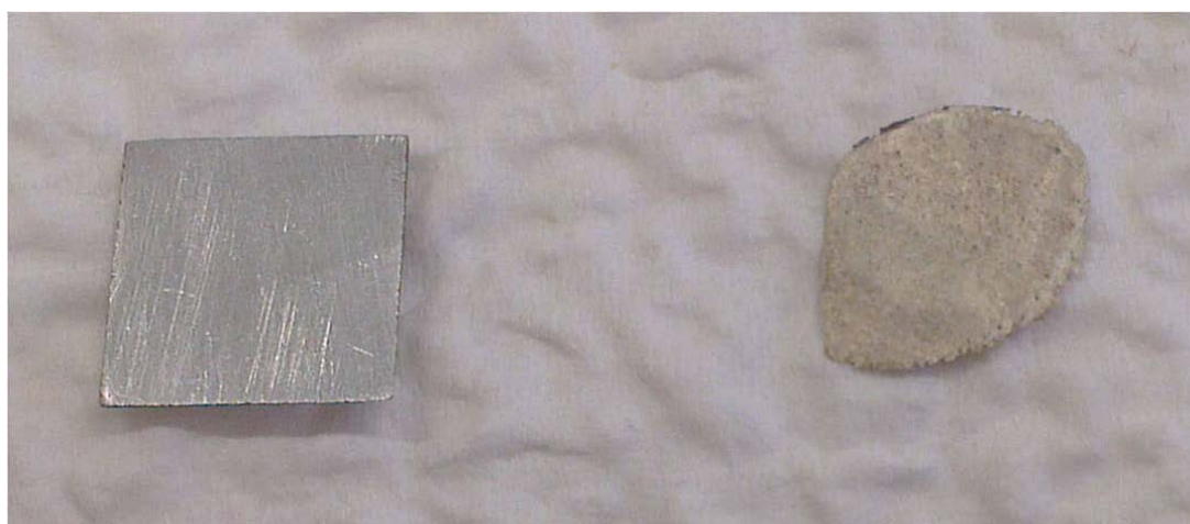
Figure 3.1: Photograph of visible difference between polished magnesium pre (left) and post (right) pH 3.0 acetic acid pre-treatment
