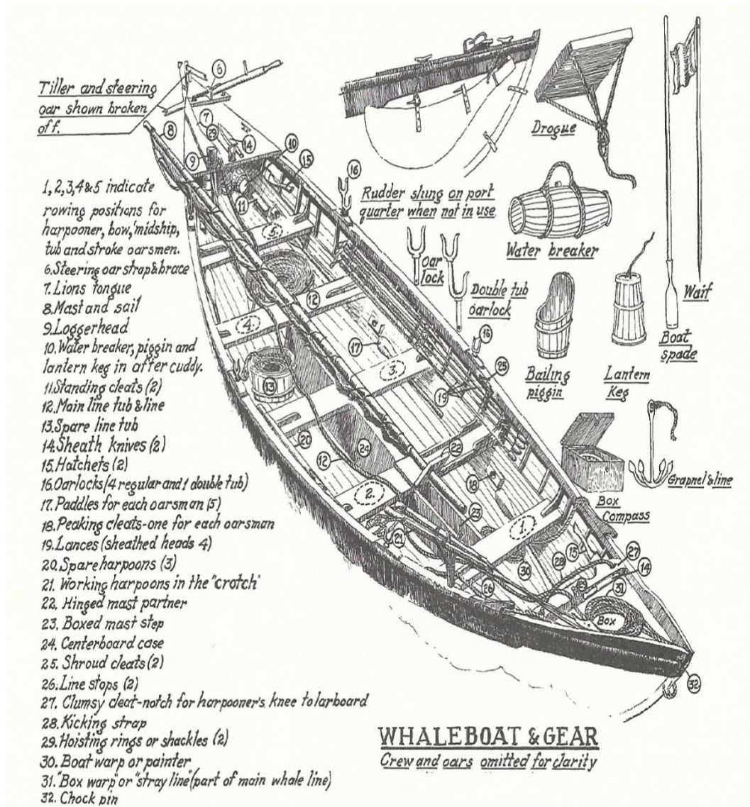
Figure 7: Diagram of a typical whaleboat and gear (Leavitt 1973).
