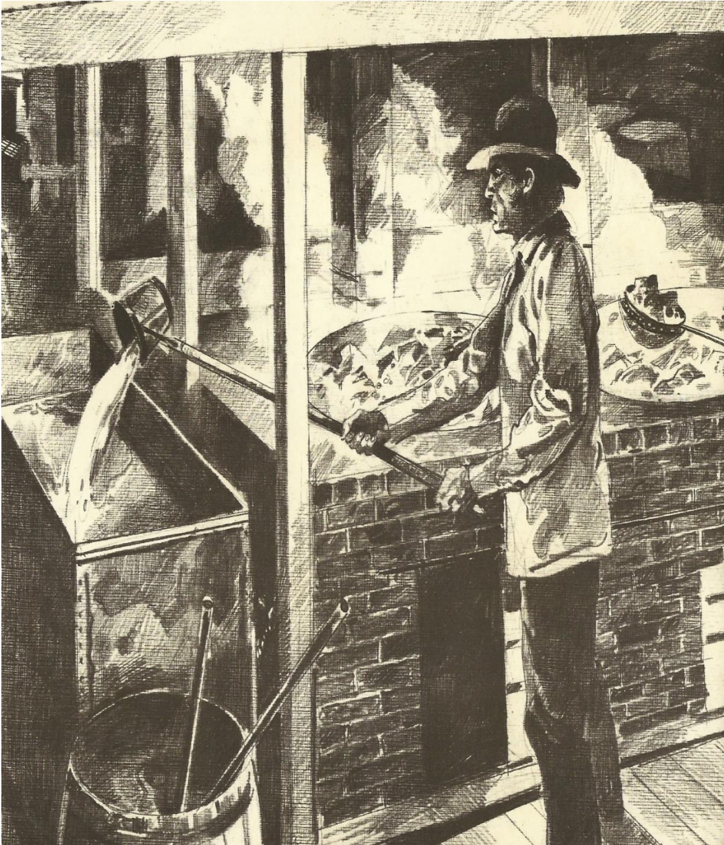
Figure 10: Image showing onboard tryworks, including the brick wall, access door and cooling tank (Whipple 1979).
