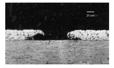
Figure 6.1 SEM image of an uncoated defect, courtesy of BlueScope Steel<sup>®</sup>.
