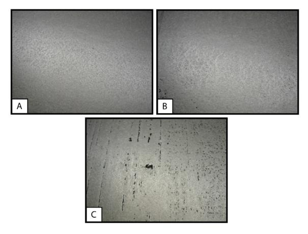
Figure 6.2 Photographs of typical defect free (A), pinhole uncoated (B) and gross uncoated (C) hot dip metallic coatings.
