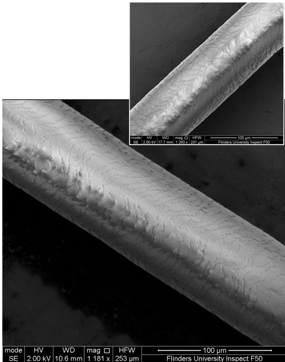
Figure 30: SEM images of healthy, untreated human scalp hair (top) and hair treated with Olaplex® incorporated into a bleach treatment (bottom). This single strand of hair was imaged before and after treatment, with the treatment taking place on the SEM stub on which the hair was mounted. Images taken using Inspect FEI F50 SEM
