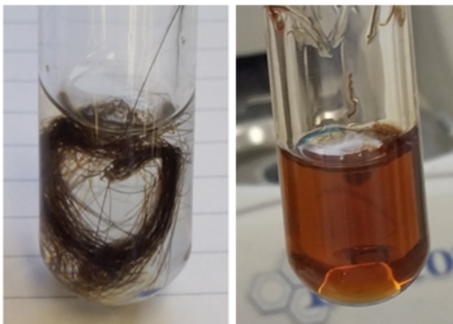
Figure 10: 20 mg of un-cut hair in 2 mL ILC, before heat treatment (left); 20 mg of un-cut hair in 2 mL ILC after being heated in an oil bath to 150 °C (right)
