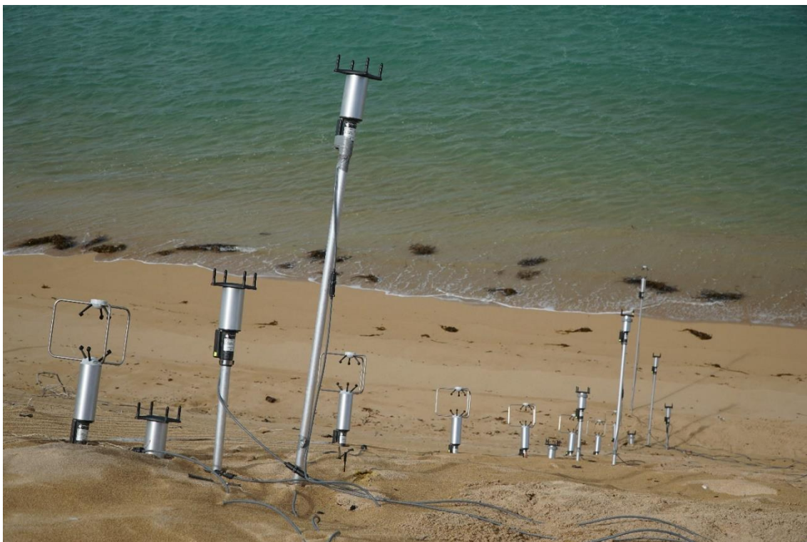
Figure 35: Experimental set up looking downslope from the 3D and 2D anemometers positioned at 18 m up the dune slope from the dune toe.
