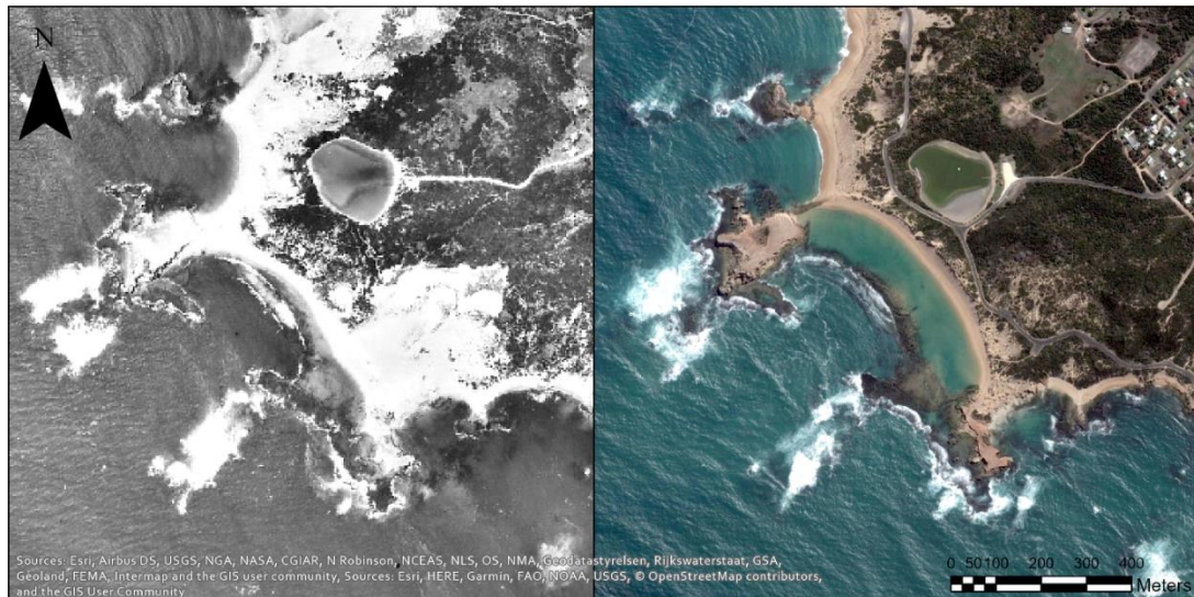
Figure 16: Aerial image of Salmon Hole taken in 1946 (left panel) and in 2016 (right panel). Severe erosion and development of a lagoon has occurred at Salmon Hole.
