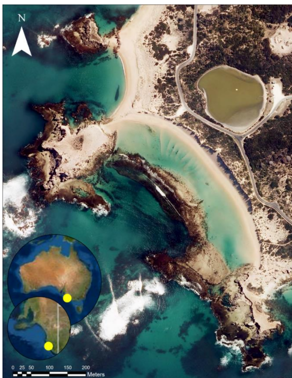
Figure 15: Salmon Hole study site situated near Beachport SE South Australia (image from 2013). The reef which extends across the bay is semi-exposed at low tide as shown in this image. A prominent scarp may be observed along the dune edge. An artificial rock 'tombolo' is present at the northern margin of the bay. The beach originally reached the seawards edge of the exposed reef in 1946.
