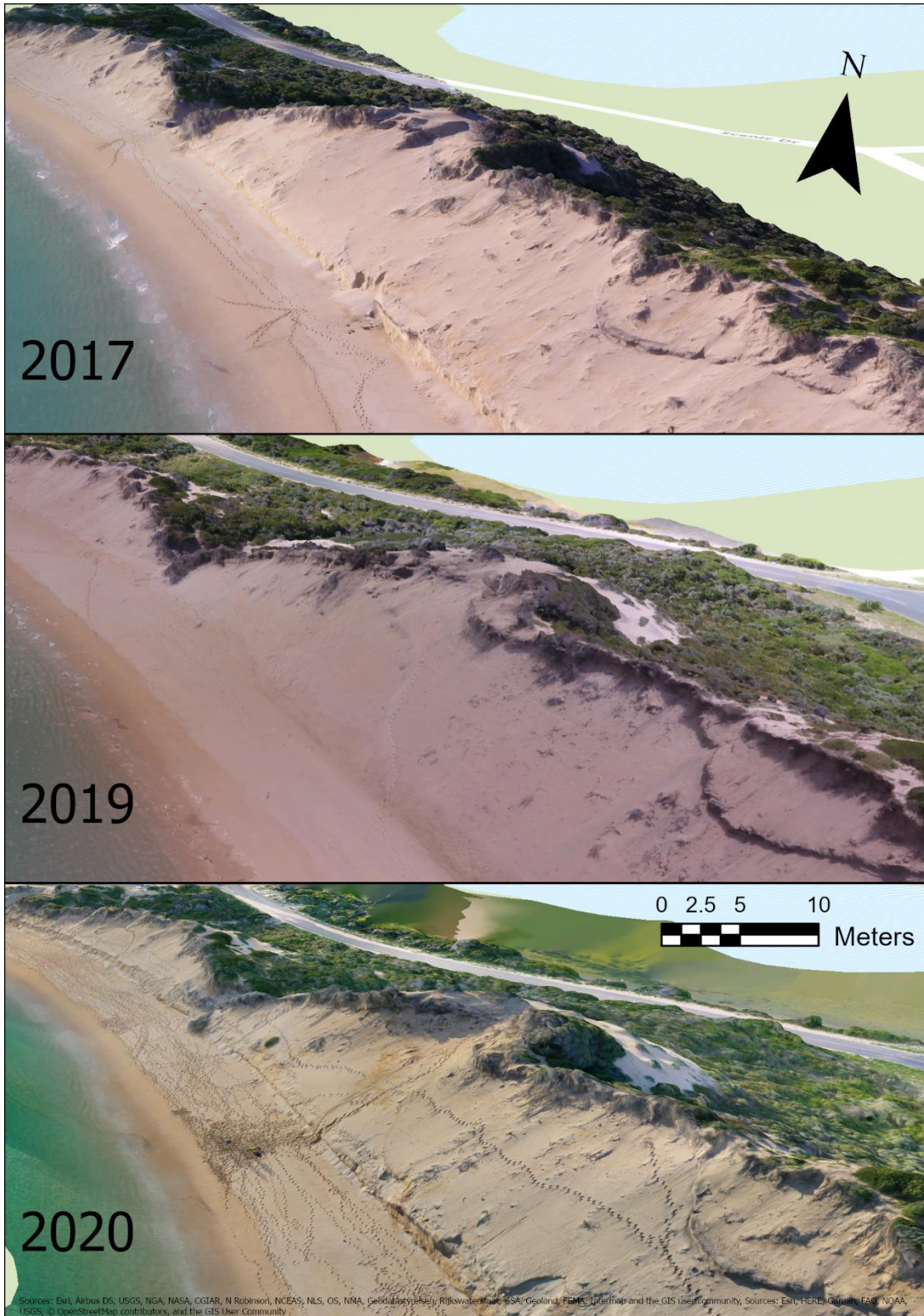
Figure 28: Oblique angle of DSM's of Salmon Hole created through drone surveys and Pix4D photogrammetry software. Surveys from 28-8-2017, 15-2-2019, and 16-5-2020 are shown. Both the survey from 2017 and 2020 show recent scarping at the base of the dune in contrast to the summer survey in 2019 where lack of storm activity has led to a completely avalanched profile. Blowout depositional lobes on the dune scarp crest have increased in size from 2017 to 2020.
