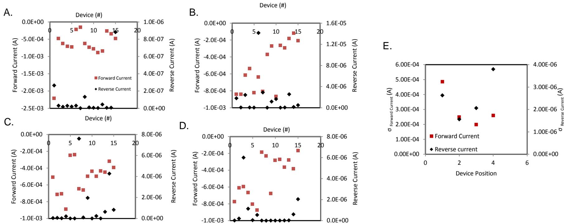
Figure 4.17. Distribution of forward current (red) and reverse currents (black) with respect to device position and the resulting standard deviation. A. Distribution of currents in position 1. B. Distribution of currents in position 2. C. Distribution of currents in position 3. D. Distribution of currents in position E. Calculated standard deviation by device position.
