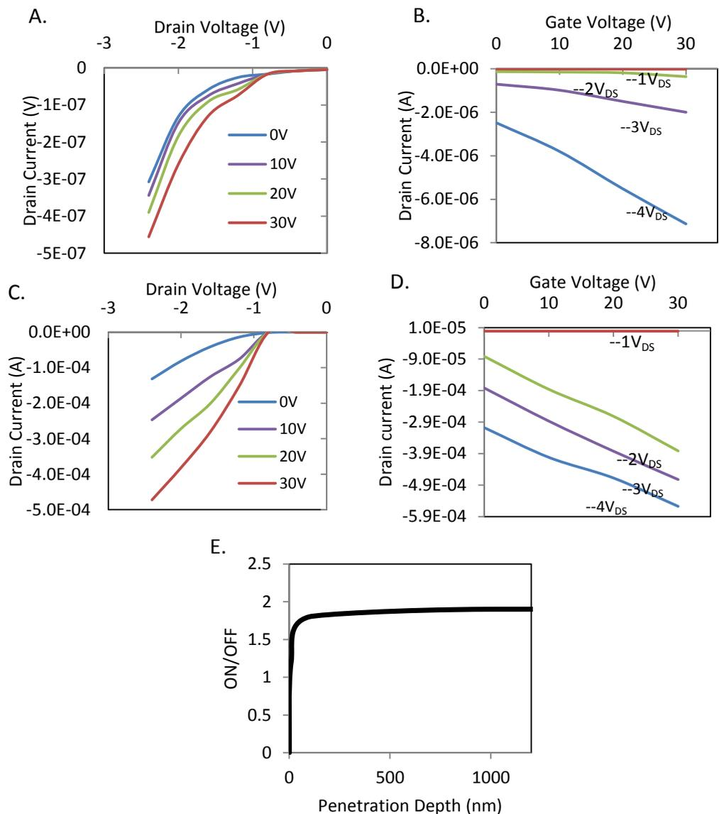
Figure 7.5. Simulated transistor performance. A. Output plot for 20 $\mu\text{m}$  active layer thickness. B. Transfer plot. C. Output plot for 225nm active layer thickness. D. Transfer plot. E. Role of penetration depth on transistor performance.
