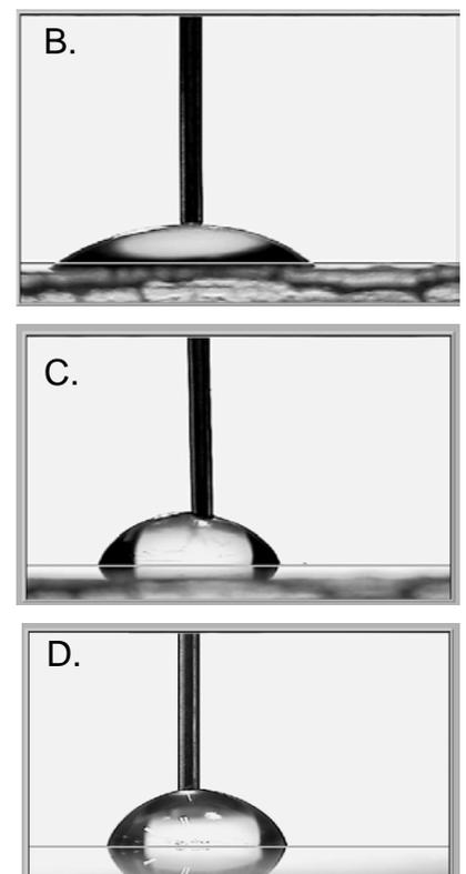
Figure A.4. Contact angle vs. time for evaporated (blue dots) and evaporated (red dots) gold samples. Example digital capture of obtained contact angle droplets for A. 1,2-DCB on cleaned Au after 30mins. B. 1,2-DCB on UV-NVS cleaned surface after 60mins C. Pyroneg cleaned UV-NVS with water D. Cleaned Au with water droplet.
