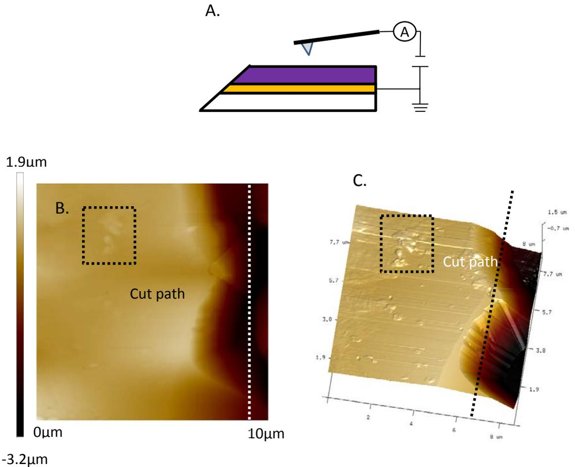
Figure 5.10 . Obtained topographic images of the cut edge A. Experimental schematic showing biases applied. B.  $10\mu\text{m} \times 10\mu\text{m}$  AFM tapping mode height image of the cut-polymer interface. C. Three-dimensional topographic image of the tapping mode two dimensional image.
