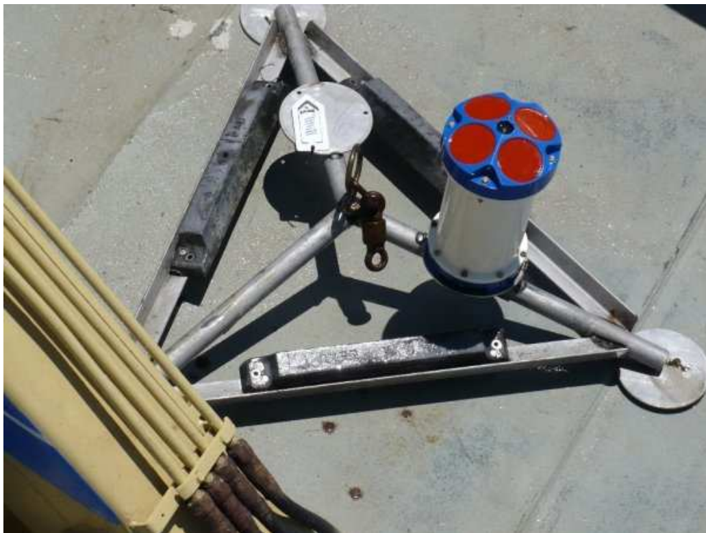
Figure 2.2: An example of the ADCP mooring used at M7, M8 and M10.
