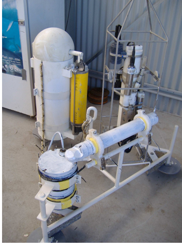
Figure 3.2: Moorings used for the collection of temperature, salinity, pressure, turbidity and currents at locations M5a and M5b (Source: CSIRO).
