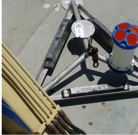
Figure 3.3: The mooring frame used to mount the RDI Workhorse (300kHz) ADCP in deployments M7 and M8.
