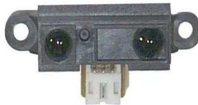
Figure 3.2: The Sharp GP2D12 infra-red sensor module. The two lenses are the emitter and the receiver of the IR beam.
