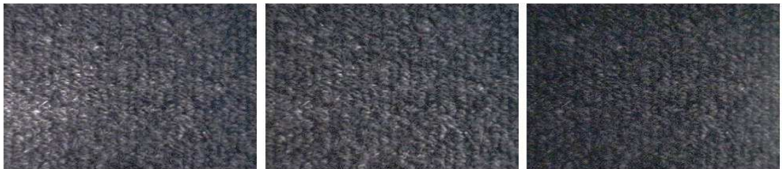
Figure 5.6: Illumination of the same carpet surface from multiple directions. The left, middle, and right image shows the carpet being illuminated from the left, top, and right respectively.
