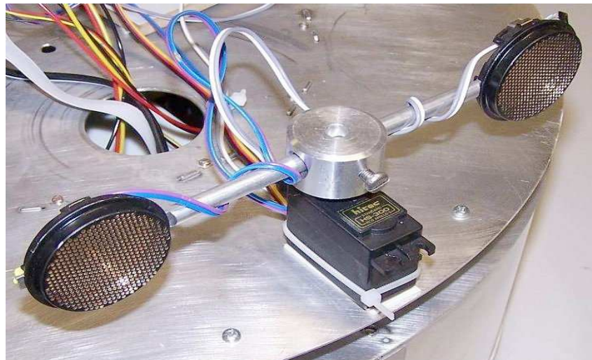
Figure 3.8: Sonar modules on top of the servo motor. The sonar sensors can be rotated independently of the robot's orientation, thus allowing greater flexibility in the sensor usage.
