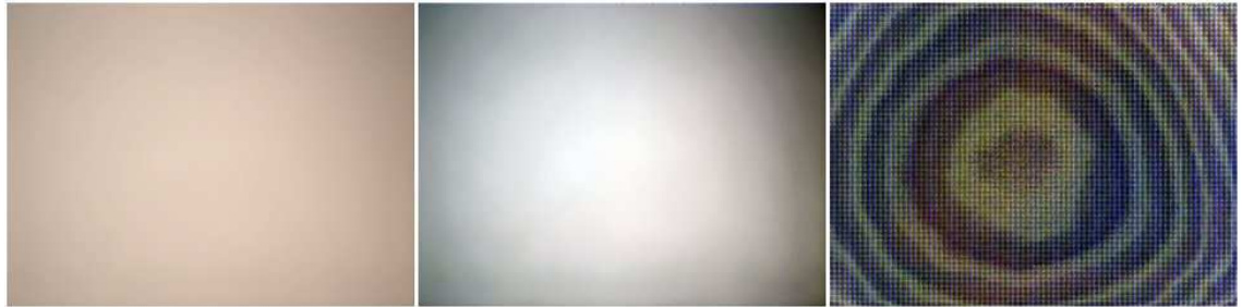
Figure 5.19: Radial shift characteristics on a uniform looking surface. Left image is the actual image captured by the camera, middle image shows the stretched image to highlight the difference in the intensity. The right image shows the standard deviation, which clearly shows the formation of bands to group the similar intensities.
