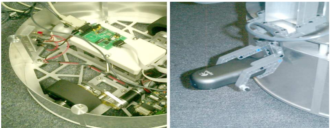
Figure 7.3: Webcams placed within and on the side of the robot. Left image shows the eyeball camera just behind the battery, while the right image shows the configuration of the side mounted camera.
