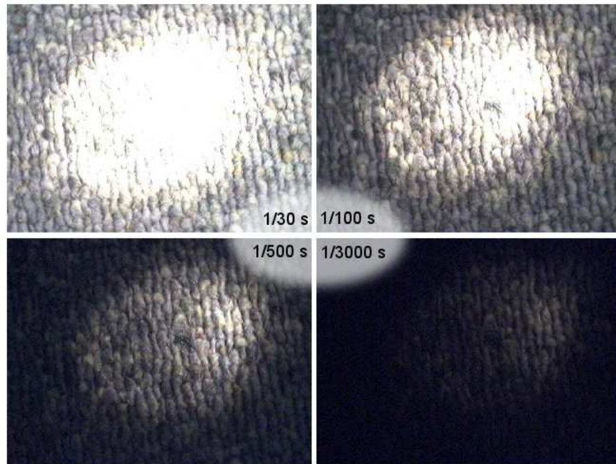
Figure 5.9: Various exposure time at constant brightness. The exposure time is decreased in the order of top left, top right, bottom left, and then bottom right.
