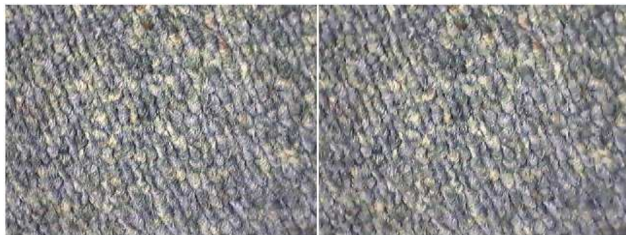
Figure 5.21: Interpolation based on threshold noise levels. The left image shows the original image, while the right image has been filtered with a selective filter which only blurs if the neighbours are of similar intensity.
