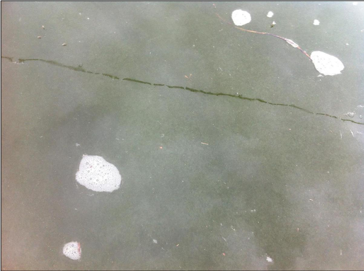
**Plate 6.7.** Visible floc formation in the Flocculation high rate algal pond at the Kingston on Murray wastewater treatment system, Australia, post-magnesium and slaked lime addition.
