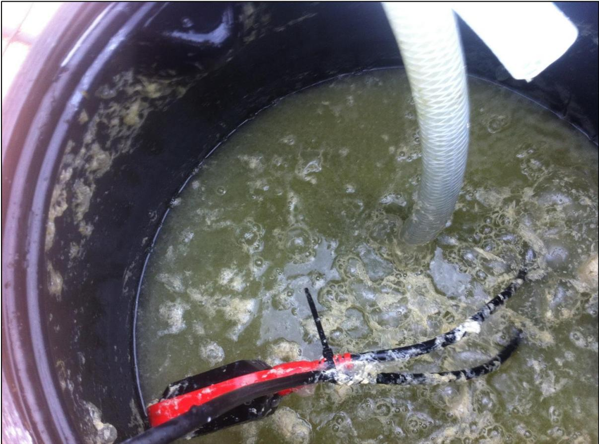
**Plate 6.6.** Visible precipitation of magnesium hydroxide and microalgae flocculation in the wastewater contained within the dosing apparatus during slaked lime addition. The wastewater was from the Flocculation high rate algal pond at the Kingston on Murray wastewater treatment system, Australia, post-magnesium addition.
