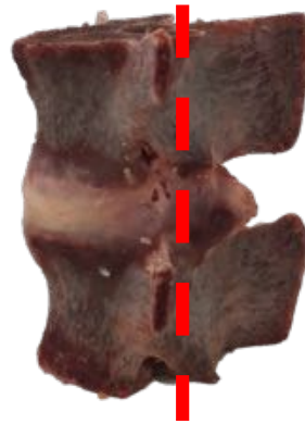
Figure 33. Lateral view of FSU. Dashed line indicates location of cut to remove facet joints
