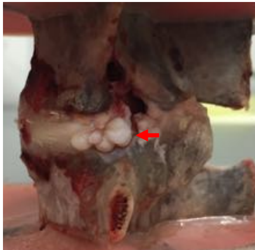
Figure 44. Left postero-lateral herniation in lateral bend (SO6). Arrow indicates nucleus extruded.
