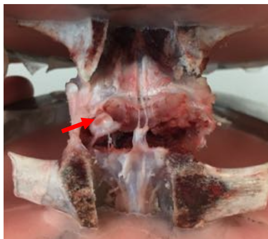
Figure 45. Posterior view of inferior endplate-vertebra fracture with nucleus extruded (arrow) in SO16 loaded in flexion and lateral bending.
