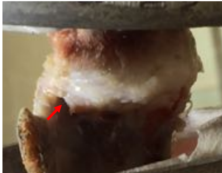
Figure 48. Image of SO23 failed at inferior endplate-vertebral interface (arrow) with no nucleus extruded. Loaded in flexion and lateral bending
