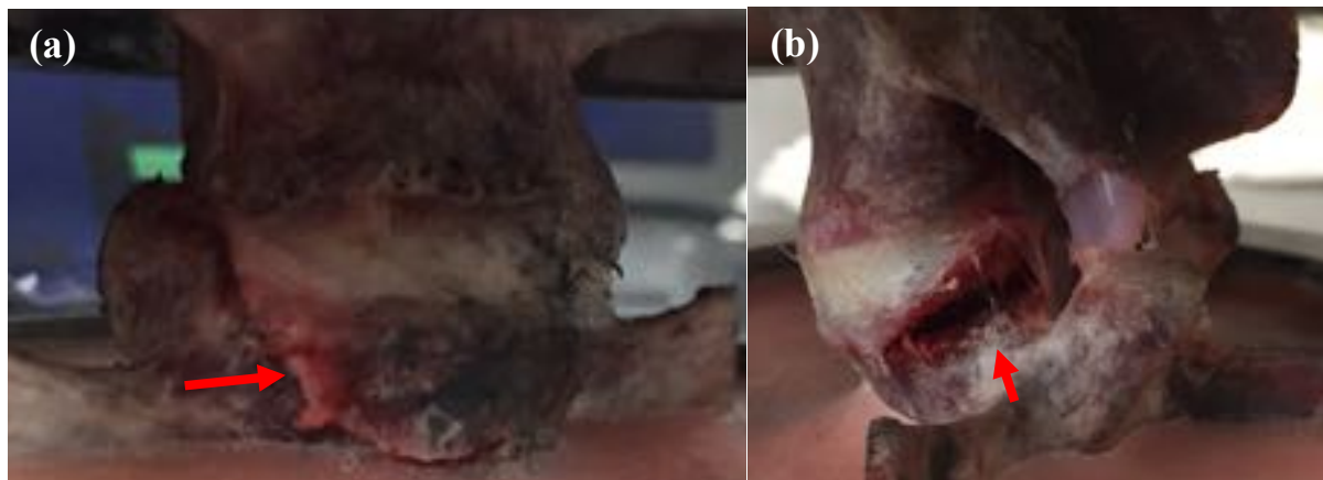
Figure 39. Images of inferior vertebral fracture in pilot test FSUs. (a) Left anterior view of SSO5 (arrow: inferior vertebral shear fracture on right side). (b) View from left side of SSO6 (arrow: endplate junction failure and left facet failure).
