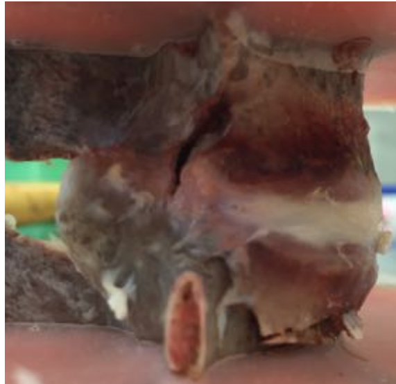
Figure 49. Image of vertebral fracture on the right side of the inferior vertebra in SO30 loaded in flexion
