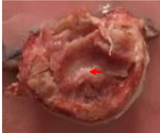
Figure 46. View of the inferior endplate of superior vertebra failed at endplate-vertebra interface with nucleus extruded (arrow) in SO27 tested in flexion and lateral bend.
