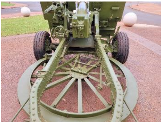
Figure 4-24: 25 pounder field artillery gun mounted on rotating ring. (located Port Hedland).
