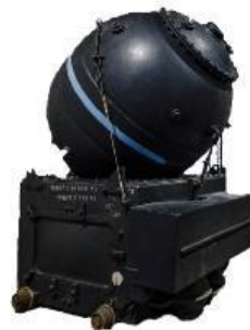
Figure 2-3: Underwater mine used at Broken Bay sitting on a mounting/anchoring platform.
