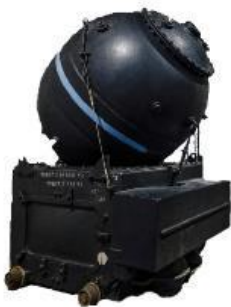
Figure 4-26: Underwater mine used at Broken Bay sitting on a mounting/anchoring platform.
