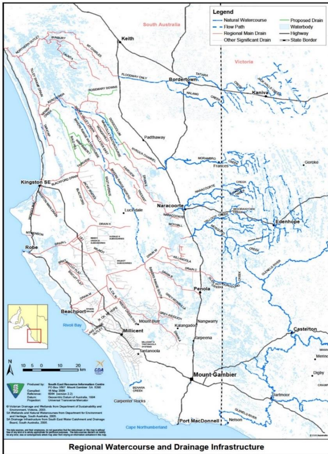
Figure 2.3: Constructed drains and natural water courses in the south east of South Australia
