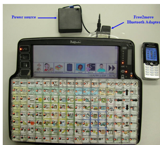
Figure 6-15 Free2move Bluetooth adapter connected to the serial port of the Pathfinder to provide wireless connection and control of the Sony Ericsson T610.
