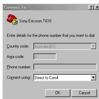
Figure 7 Connection using an unused COM port.
