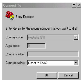
Figure 5 Connection using an unused serial COM port.
