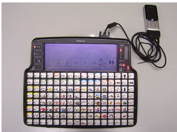
Figure 6-13 Sony Ericsson T610 to the Pathfinder via serial cable.
