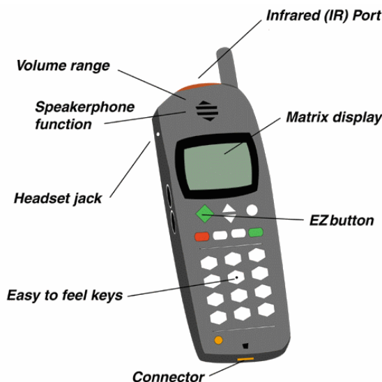
Figure 2-1 Trace Centre Reference Design 1 of a mobile phone that incorporates accessibility features (Trace Center, 2002)
