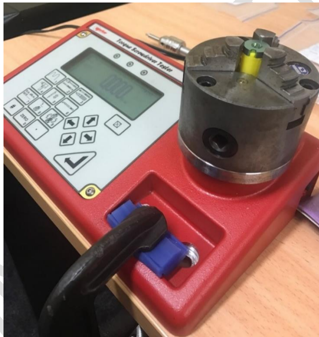
Figure 33 Norbar Torque Tester set up for screw insertion
