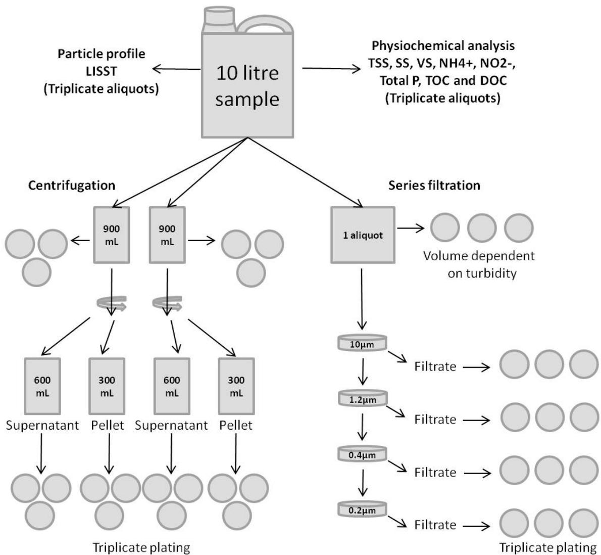
**Figure 4.1 Schematic of the two partitioning methods used**
