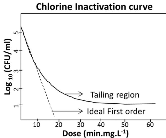
Figure 1.13 Typical Chlorine inactivation Graph
