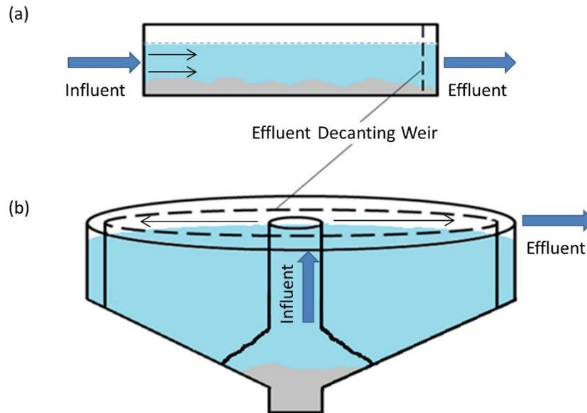
**Figure 1.3 Wastewater sedimentation tanks**
