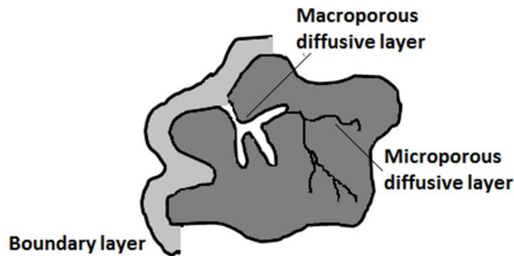
Figure 1.12 Wastewater particles structural pathways
