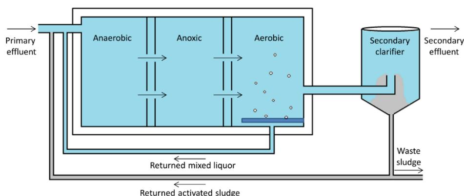
**Figure 1.4 Modified Activated Sludge**
