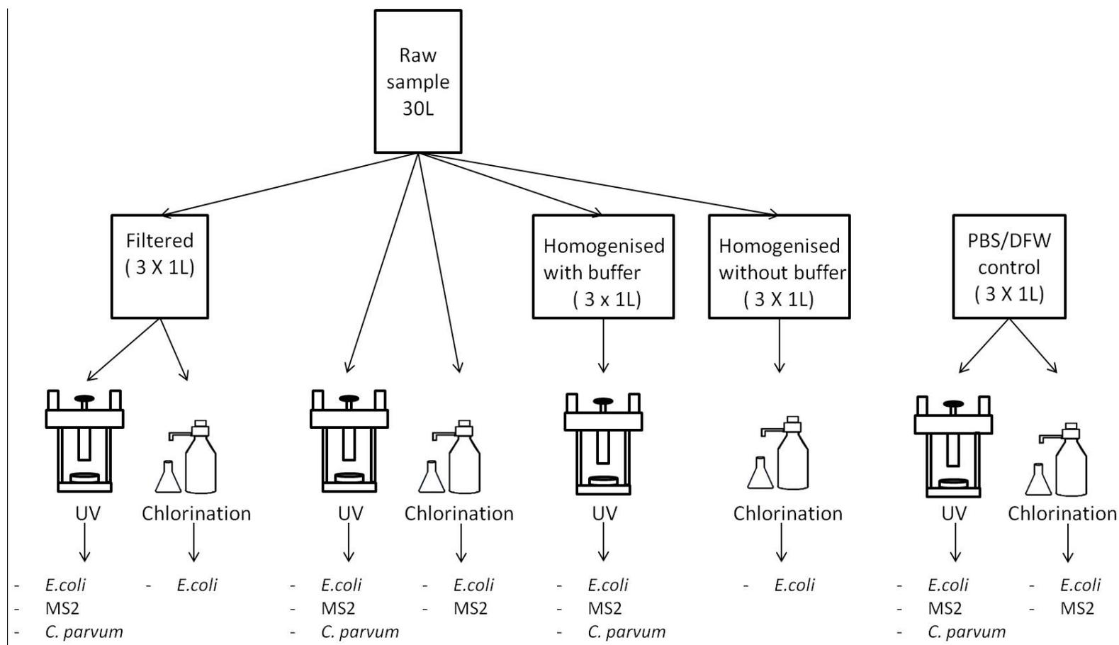
Figure 6.1 Schematic for disinfection experiments.
