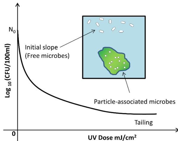
Figure 1.14 Typical UV inactivation curve
