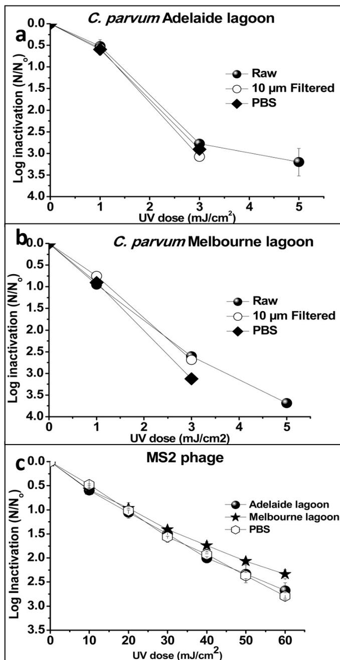
Figure 6.3 U.V Disinfection of *C. parvum* oocysts and MS-2 phage
