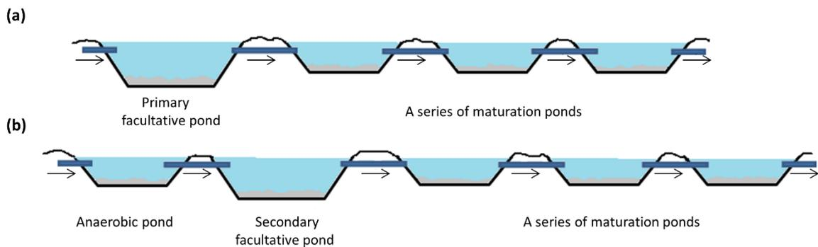
**Figure 1.5 Waste stabilization ponds**
