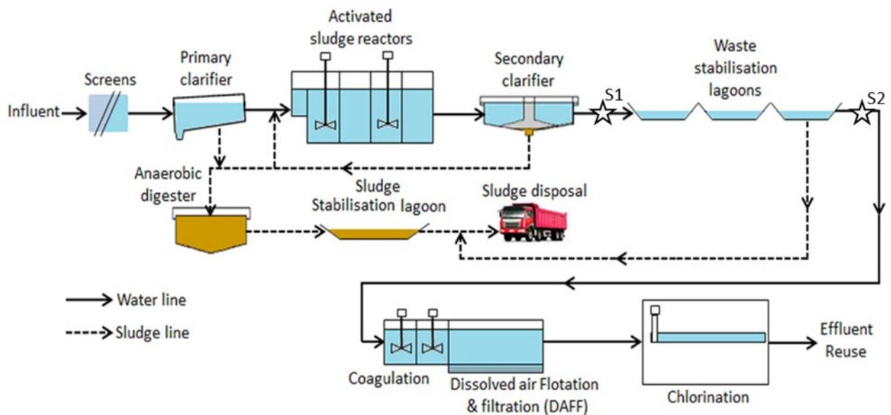
Figure 2.1 Schematics of Bolivar wastewater Treatment Plant
