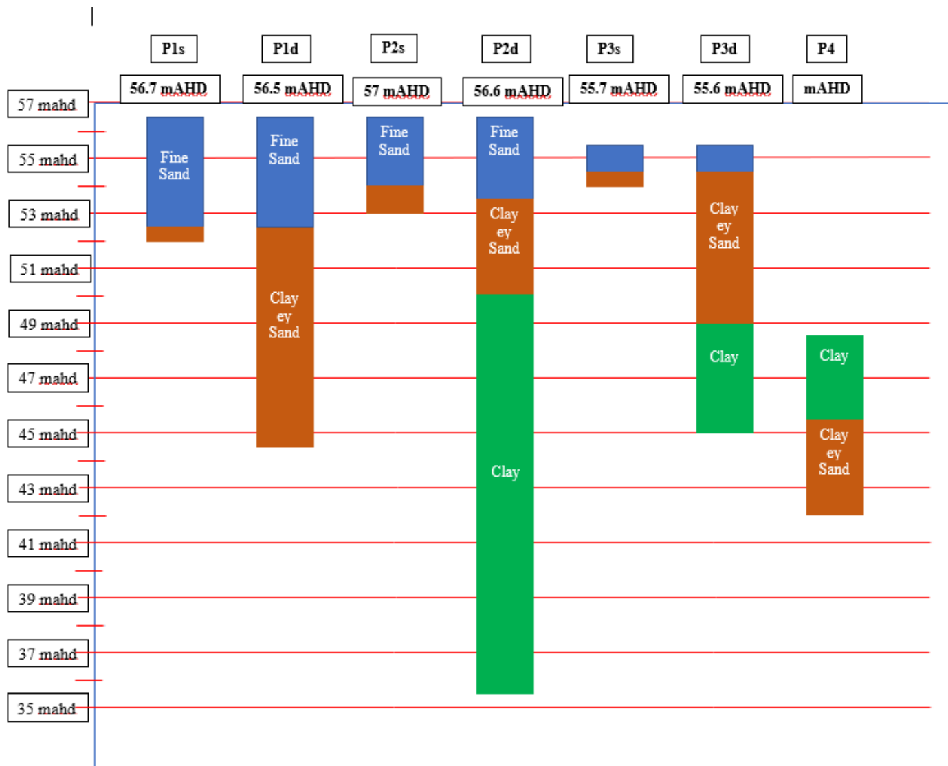
Figure 5-3: Lithological logs of the seven piezometers located in the study area parallel to the ERT transect
