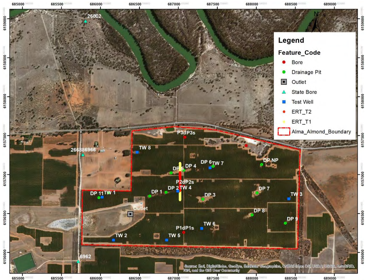
Figure 4-1: ERT survey transects and water monitoring infrastructure (piezometers, test wells, drainage pits & state groundwater bores) in the study area. The detail of ERT transects is in Section 4.2.1.2. Drainage pits and outlets are described in section 4.2.3. Test wells, piezometers and state bores are described in Section 4.2.4.
