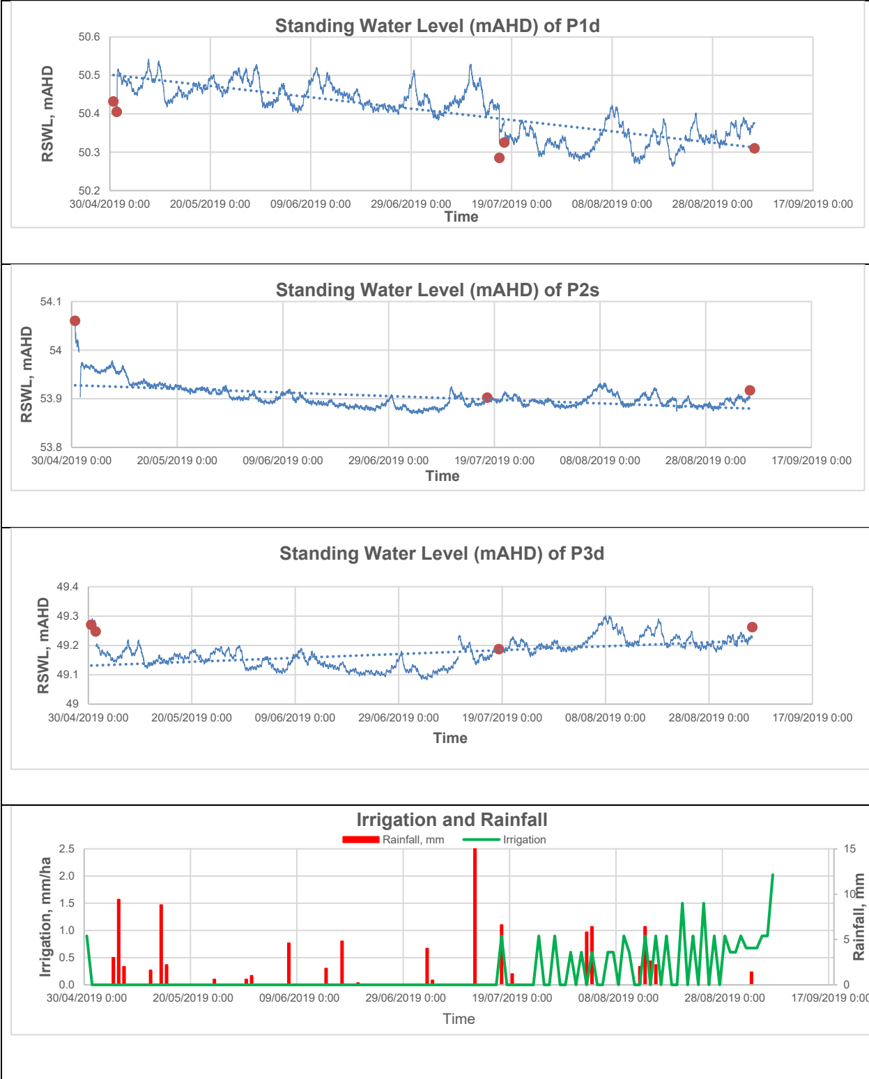
Figure 5-17: Reduced standing water level (RSWL) (mAHD) in piezometers from 30 April to 3 September 2019.
