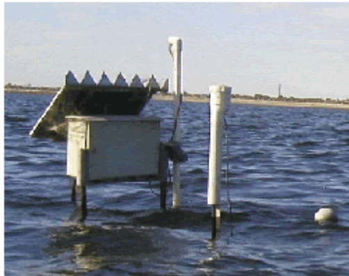
Plate 4.4. Installed handmade online monitoring station showing solar panel and bird deterrent on upper edge. A temperature probe station is located in the foreground. The buoy to the lower right of the image supports the temperature thermistor chain at this location (Location I).
