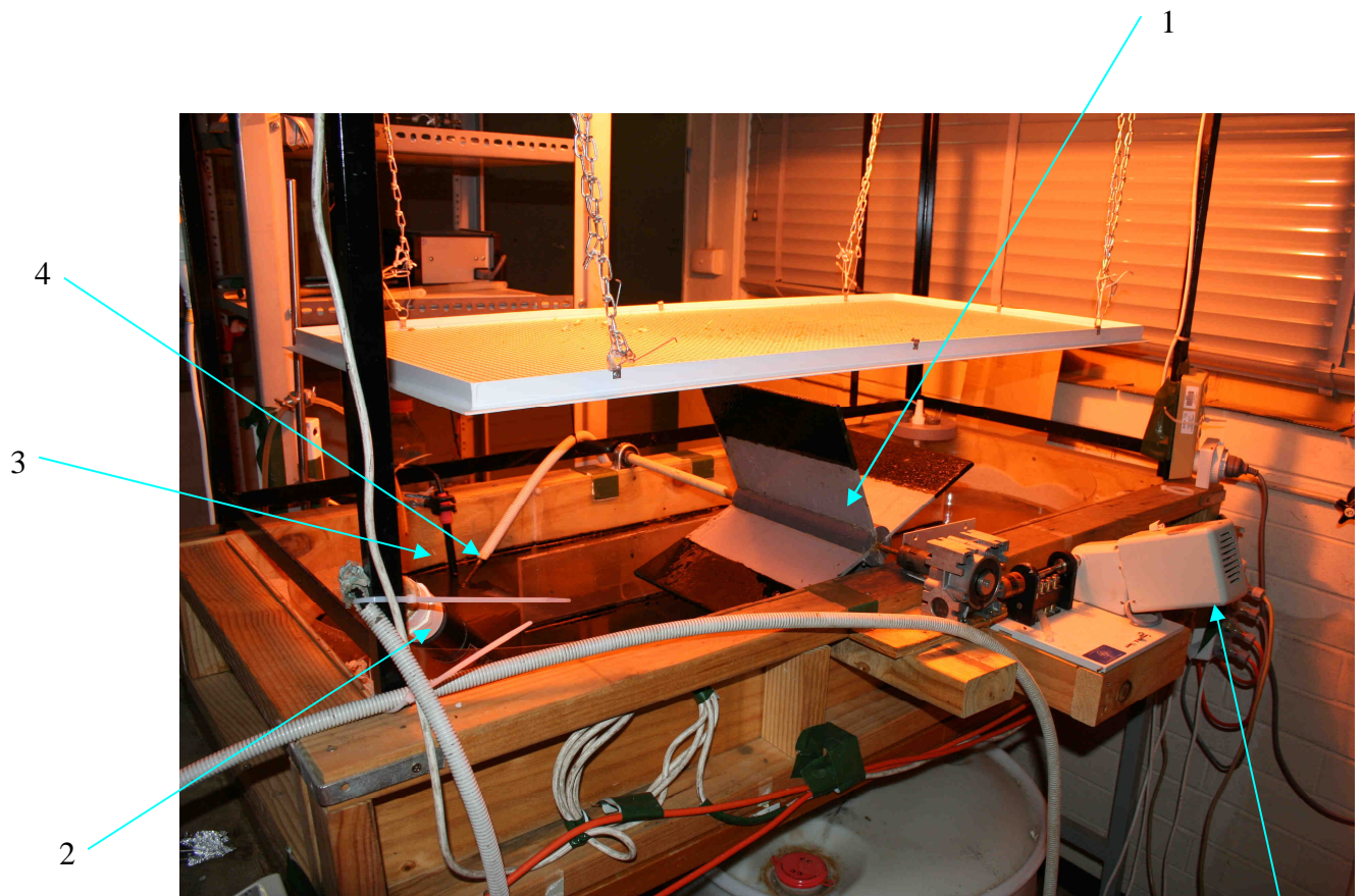
Plate 4-2. HRAP Bioreactor. Paddle Wheel (1), Dissolved Oxygen Probe (2), pH Probe (3), Temperature Probe (4), Variable Speed Drive (5).
