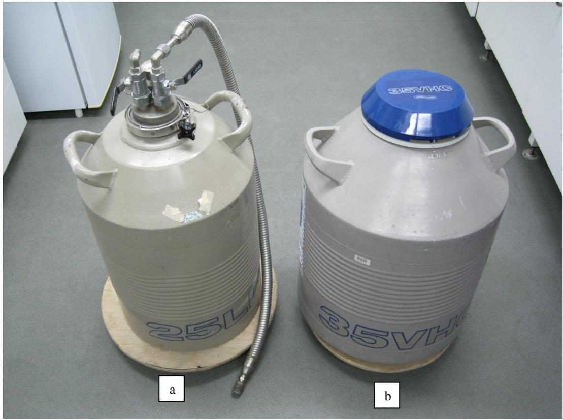
Figure 2. a) liquid nitrogen transportation dewar and b) liquid nitrogen storage dewar.
