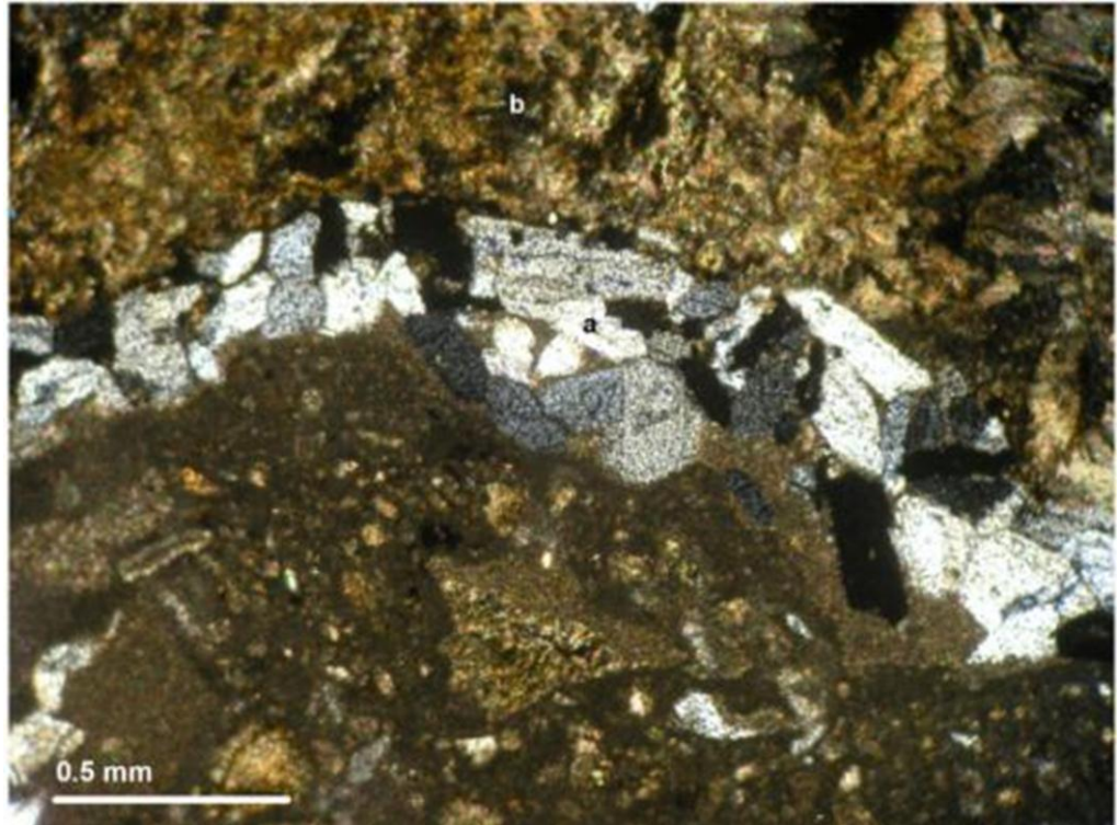
Photo 3: Euhedral gypsum crystals (a) in carbonate mud and micrite-fracture fill. Crystals show geopetal depositions, being deposited on the edge of the fracture. Illite matrix of shale evident at top of image (b). Crossed polars.
