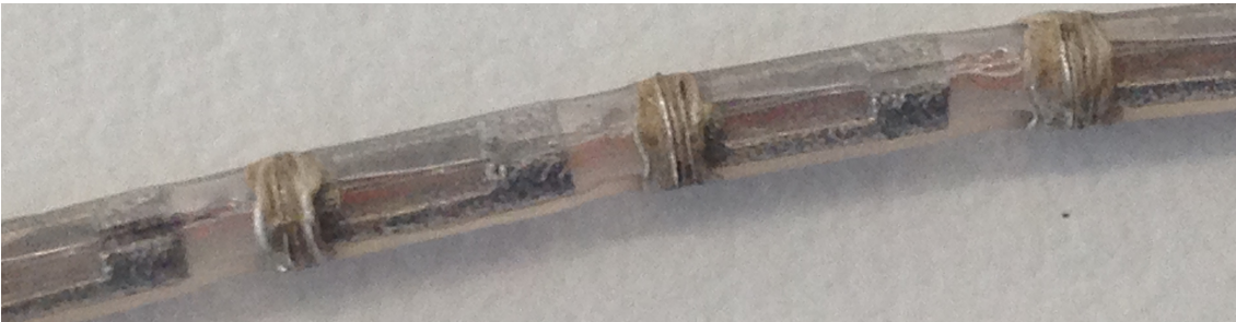
Figure 4.3: (a) Schematic of a section of the impedance manometry catheter showing the location of optical fibre sensors, electrical wires, electrodes and dual lumen extrusion. (b) Catheter assembled with electrical wires wrapped around the lumen. (c) Silver electrodes formed by silver-conductive epoxy.
