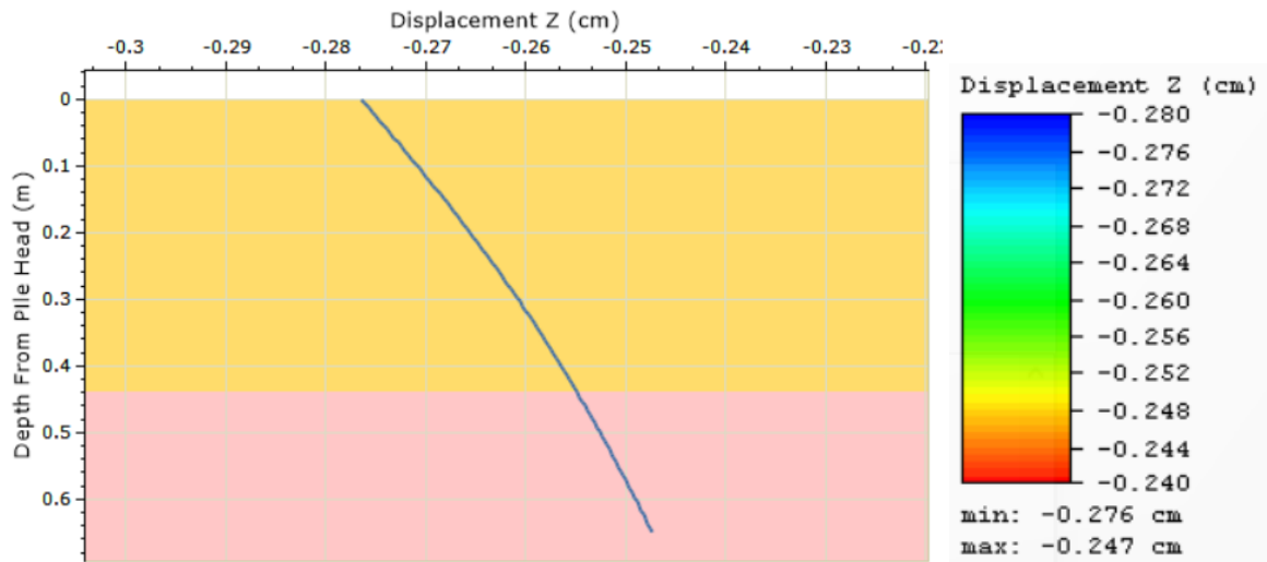
Figure 32. RSpile model-Case study 1 ( P = 2.9 \text{ kN} )-Displacement
