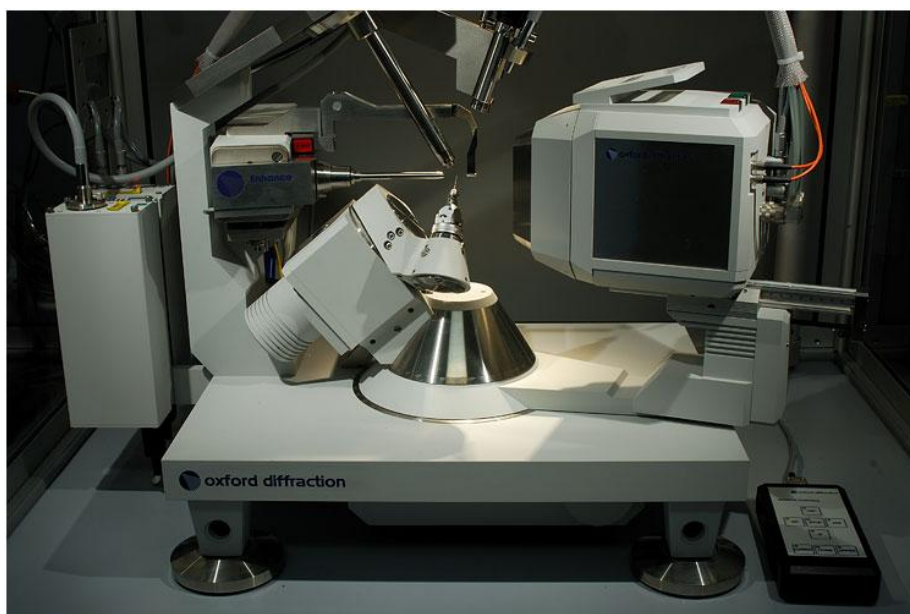
Fig 17. A Mo-target Oxford Diffraction X-Calibur X-ray diffractometer for small molecule structure determination. This image was taken in the Bragg crystallography facility at Adelaide University (SA).
