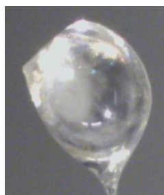
Fig 61. A sample of 34a loaded onto a loop in Paratone-N® oil. The image was captured on the X-Calibur video microscope at Adelaide University.
