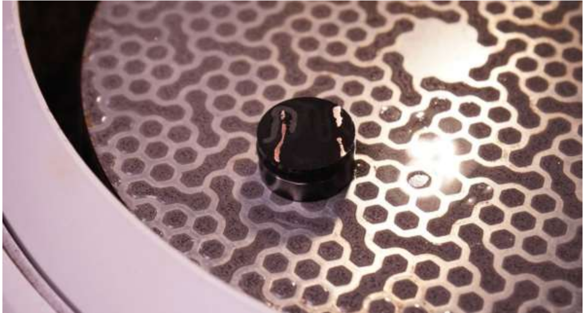
Fig. 4. Shah Muncher sample of strap embedded in a black-coloured resin mount, Sample 1156, after polishing. Photograph by Mike Ng.
