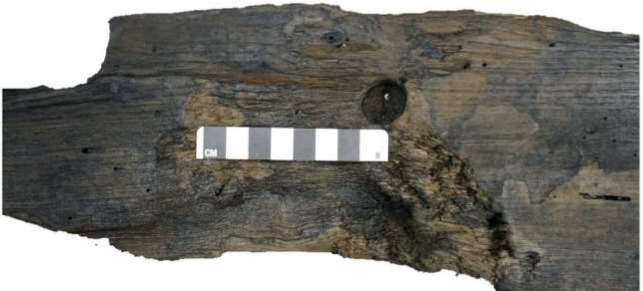
Figure 41: Close up of the treenail on PB2_904 (M. Ng, 2022).
