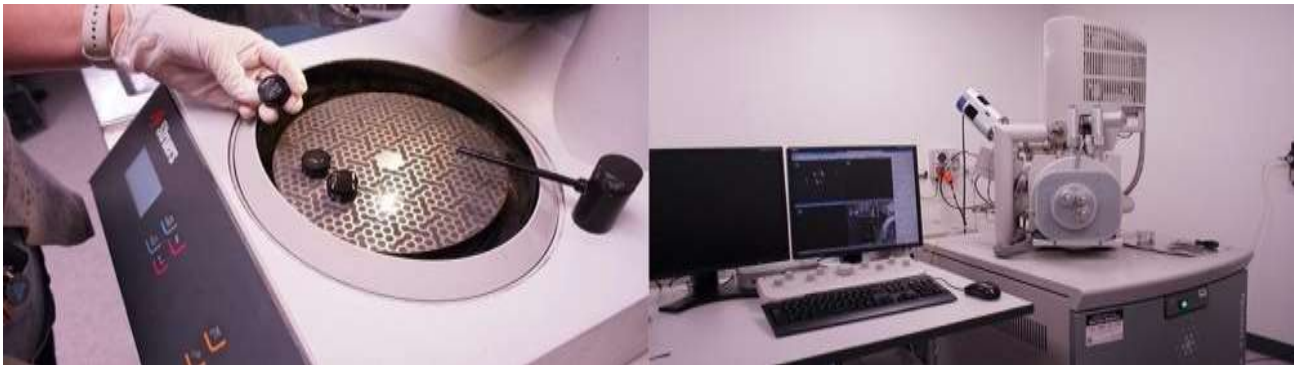
Figure 16: Samples were polished using the Struers TegraPol-11 diamond polisher (Left) before they were analysed using a FEI Quanta 450 SDD EDS detector (Right) (M. Ng, 2022).
