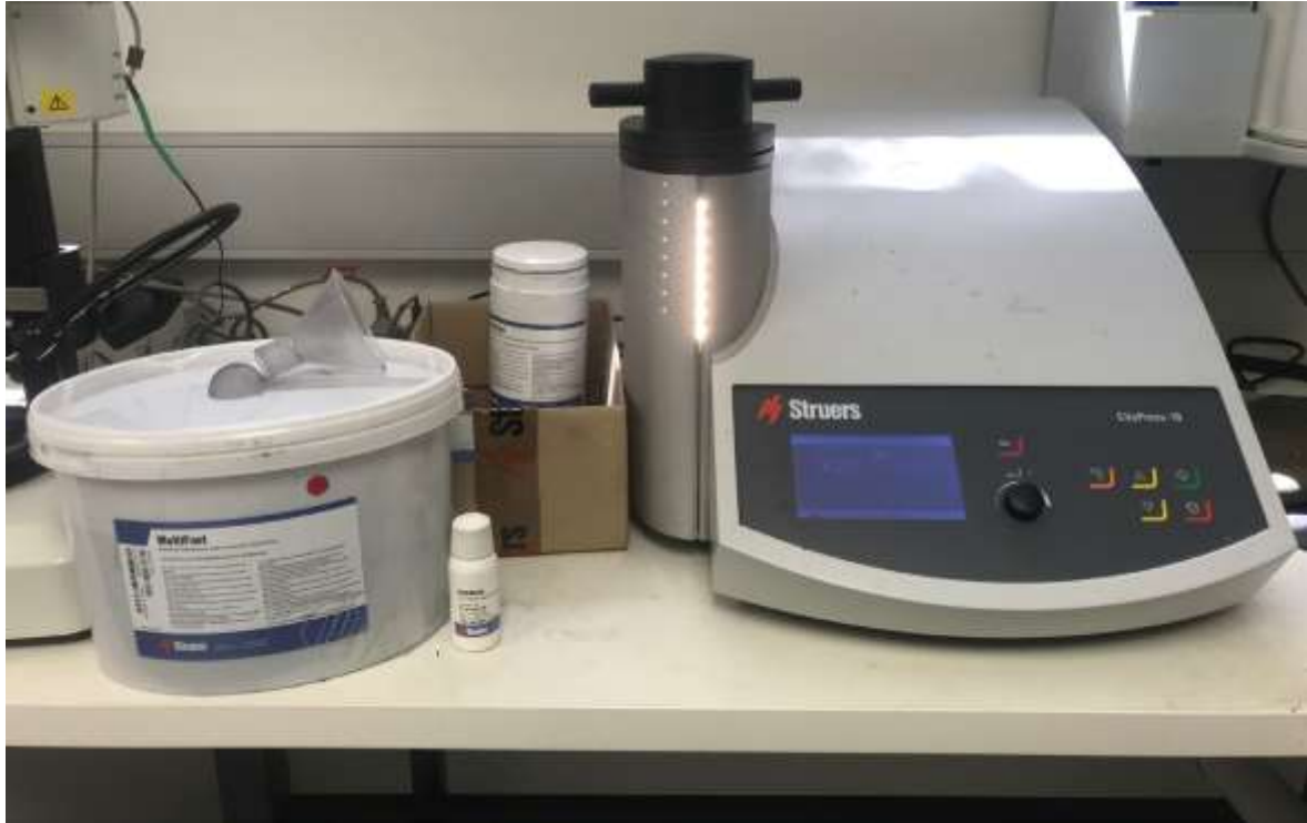
Fig. 2. Struers CitoPress-10 hot mounting press. Photograph by Wendy van Duivenvoorde.
