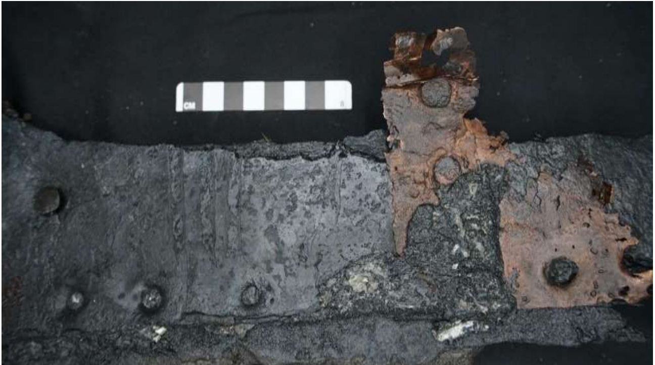
Figure 35: Section of PB2_971 sheathing where sample was retrieved (M. Ng, 2022).
