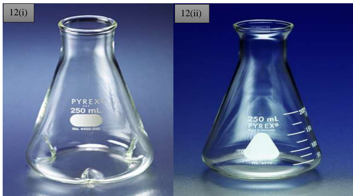
Fig.12. (i) and (ii) represents the difference between baffled and unbaffled flask.
