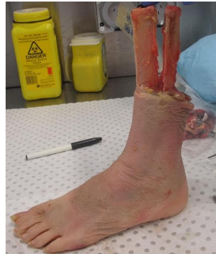
For adequate tibia potting fixation, 70cm of tibia must be exposed with all soft tissue removed.
