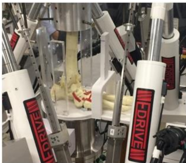
Figure 24: Hexapod Robot Simulating physical characteristics of flatfoot in sawbone model
