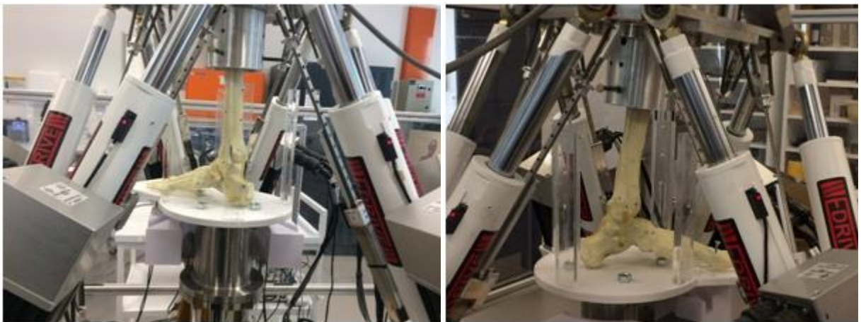
Figure 21: Hexapod Robot simulating basic flexion and extension of a sawbone model foot (Dorsiflexion and Plantarflexion)
