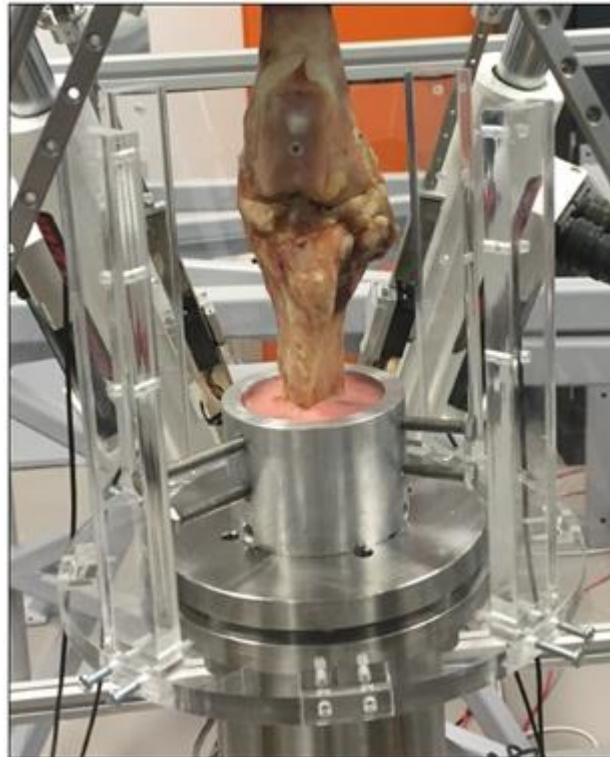
Figure 25: RSA Calibration frame for measuring ACL strain in Sheep knees Retrieved from Garcia, M., 2015. Identification of ACL strain during complex movements. Flinders University, South Australia.
