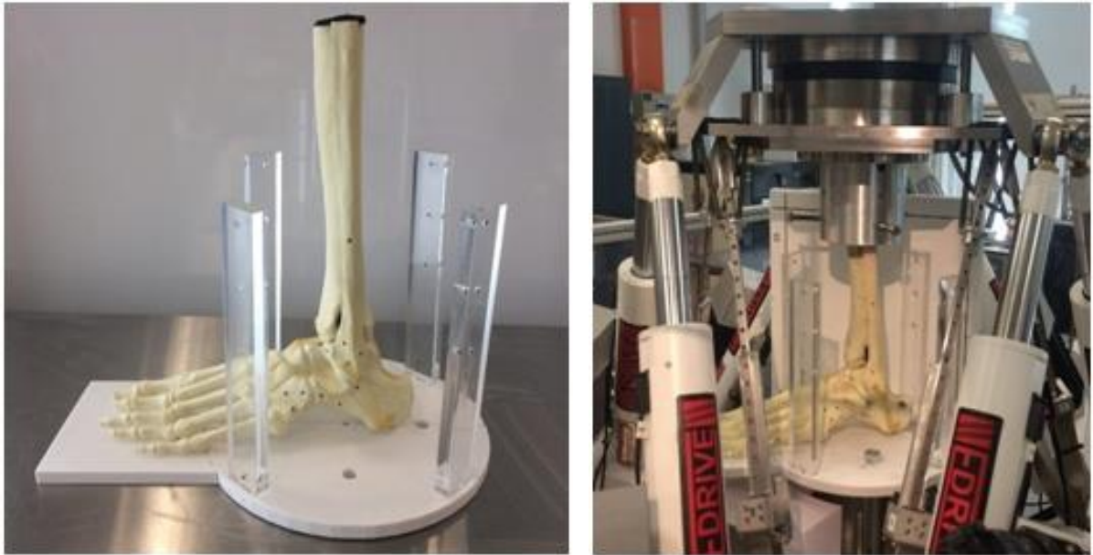
Figure 27: Concept base plate calibration cage design with sawbone foot model
