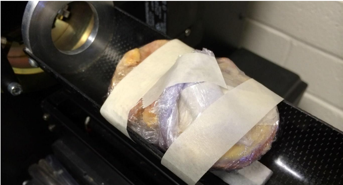
Figure 3.1: A photograph of two excised tibial plateaus, wrapped in plastic film and fixed on the carbon scanning bed of the micro-CT.
