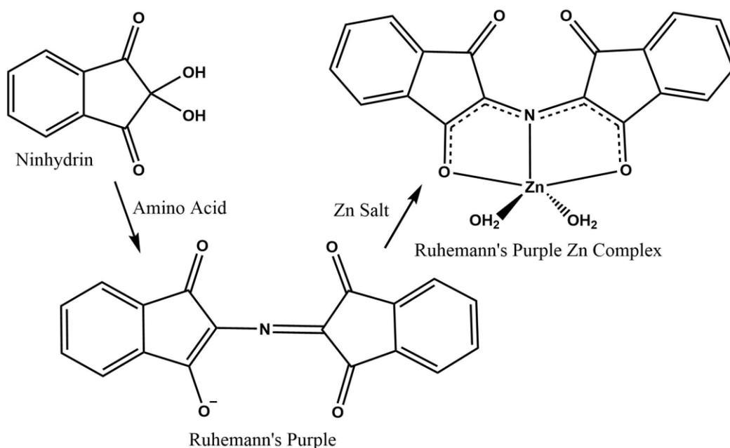
**Figure 31: The structures of ninhydrin and Ruhemann's purple along with the zinc/Ruhemann's purple complex (adapted from reported structures by Davies et al.[85] and Champod et al.[86])**
