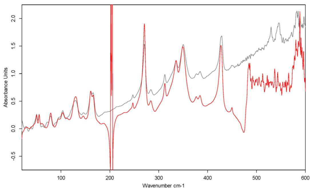
**Figure 15: Absorbance spectra for ninhydrin in PE (Grey) and PTFE (Red)**
