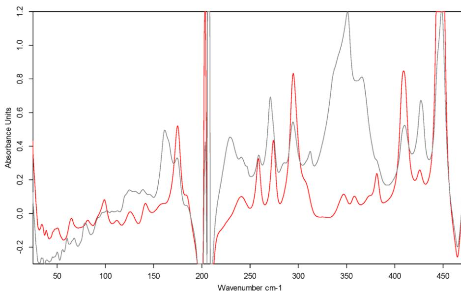
**Figure 30: Spectra of riboflavin (red) and of a mix of all three compounds (grey)**
