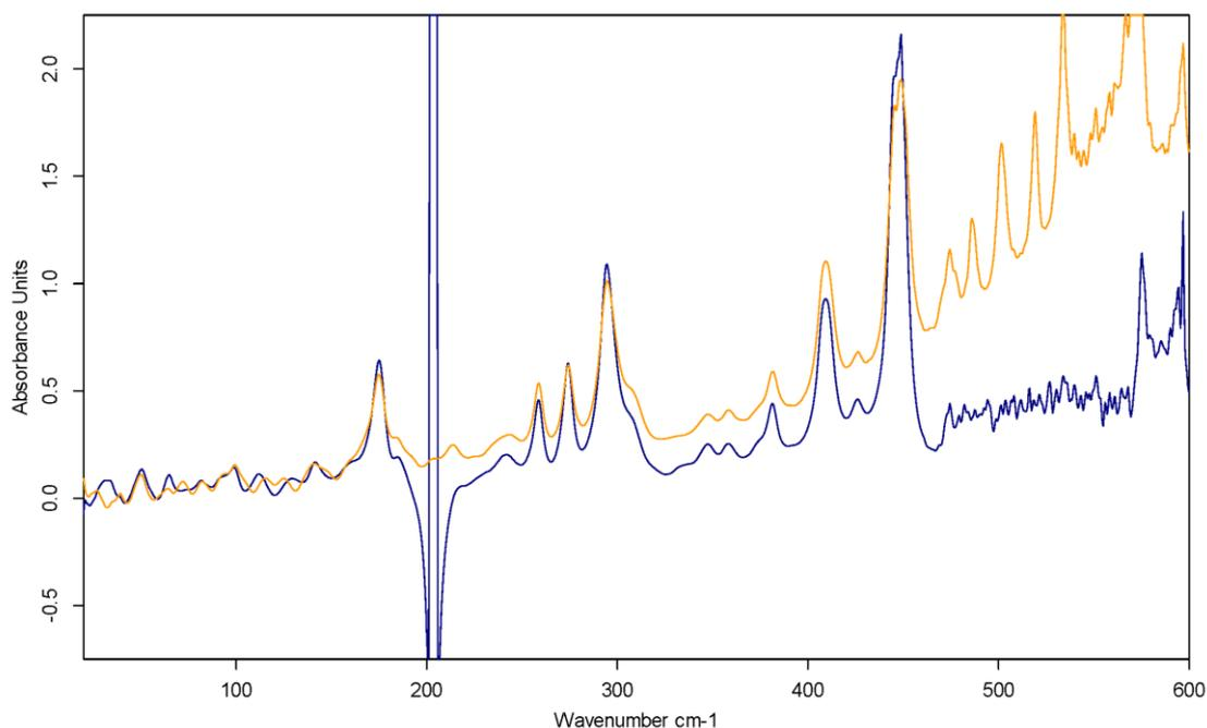
**Figure 16: Absorbance spectra for riboflavin in PE (yellow) and PTFE (blue)**
