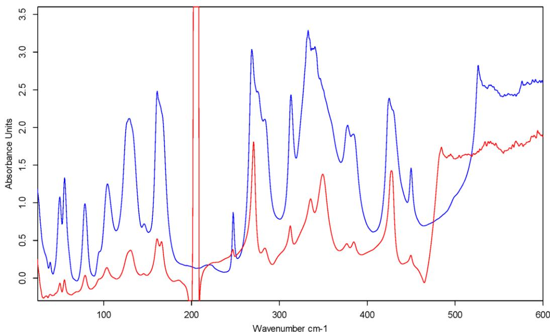
**Figure 20: Spectra for pure ninhydrin (blue) and ninhydrin in PTFE (red) overlaid**
