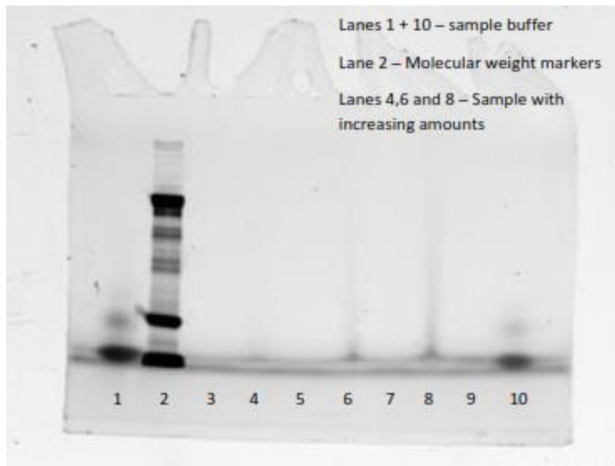
**Figure 55 Fluorescence image (488nm excitation, 610 emission) of the native gel**
