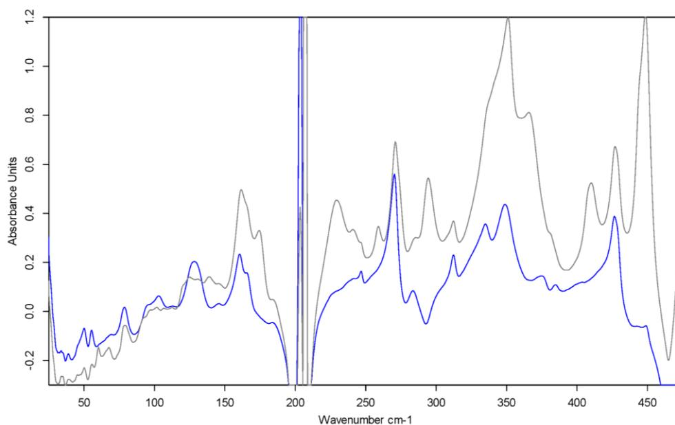
**Figure 29: Spectra of ninhydrin (blue) and of a mix of all three compounds (grey)**
