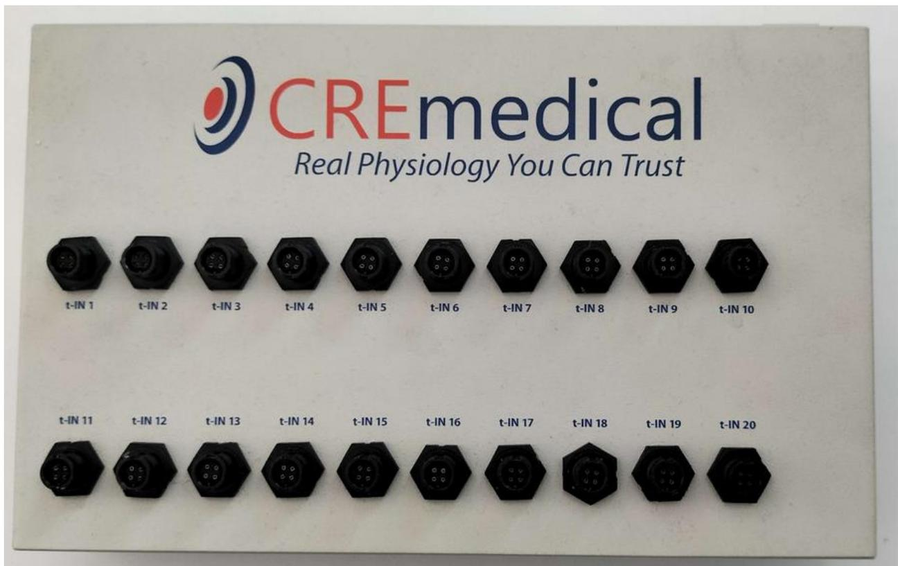
**Figure 3 The CREmedical t-interface 20. 13 tCRE electrodes were connected from the participant into this interface, which interfaced with g.tec 64-channel connector box. Each tCRE electrode produced two outputs; an emulated EEG output generated from the outer electrode ring, and a tCRE output.**
