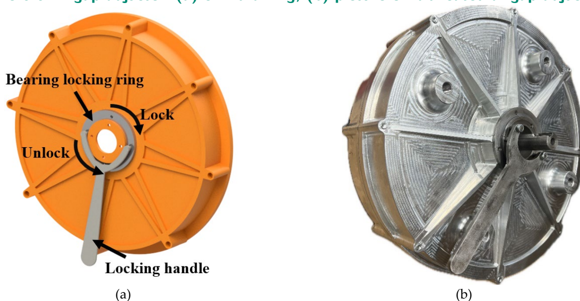
Figure 6-10 Airgap locker: (a) 3-D drawing, (b) picture of fabricated airgap locker.
