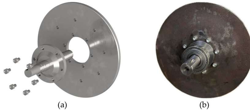
Figure 6-6 Shaft and rotor holder, (a) 3-D drawing proposed shaft and rotor holder, (b) picture of fabricated shaft and rotor holder.
