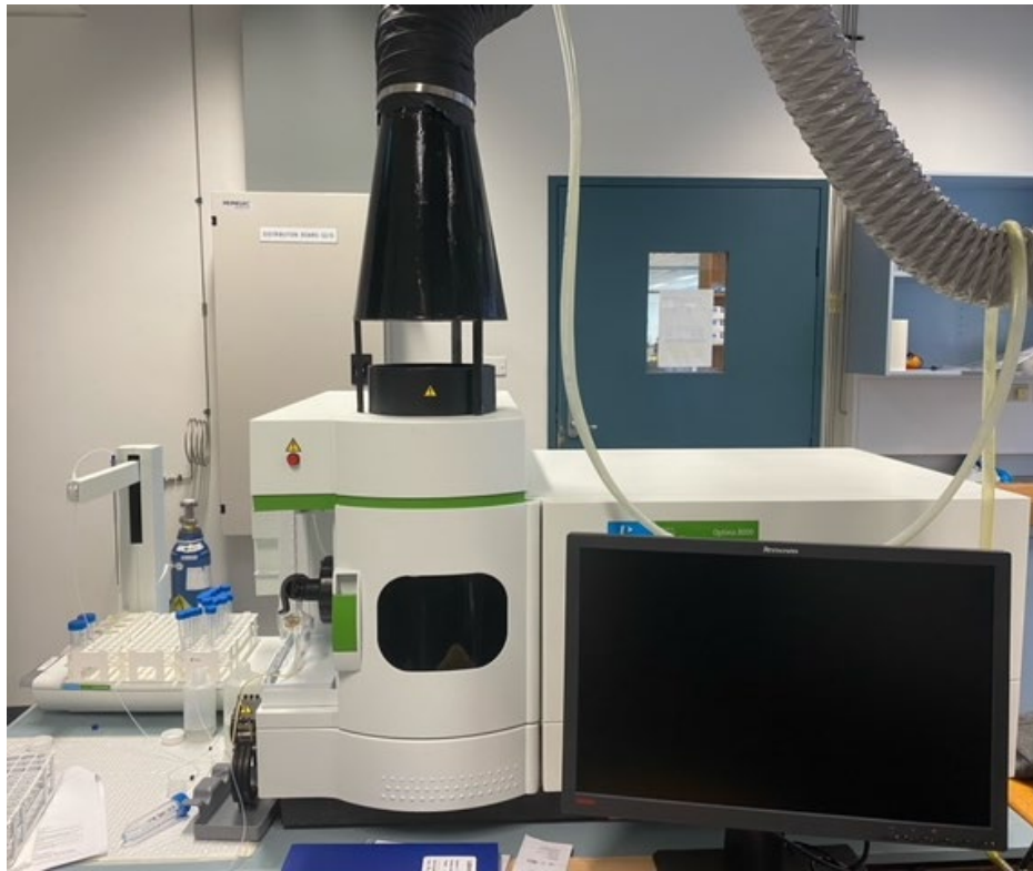
Figure 26 Inductively Coupled Plasma Optical Emission Spectrometry in Flinders Analytical (PerkinElmer Optima 8000).
