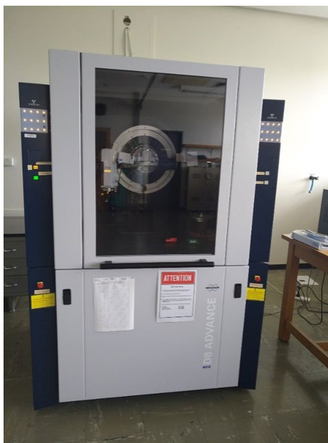
Figure 21 X-ray diffractometer in Flinders Microscopy and Microanalysis (FMMA) (Bruker, Eco D8 Advance).
