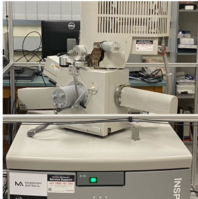
Figure 24 Field Emission Scanning electron microscope in FMMA equipped with EDAX, BSE and SE detector. (Inspect F50)
