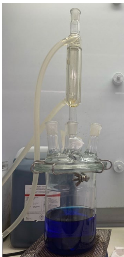
Figure 15 The reactor used in covellite leaching experiments equipped with condenser.
