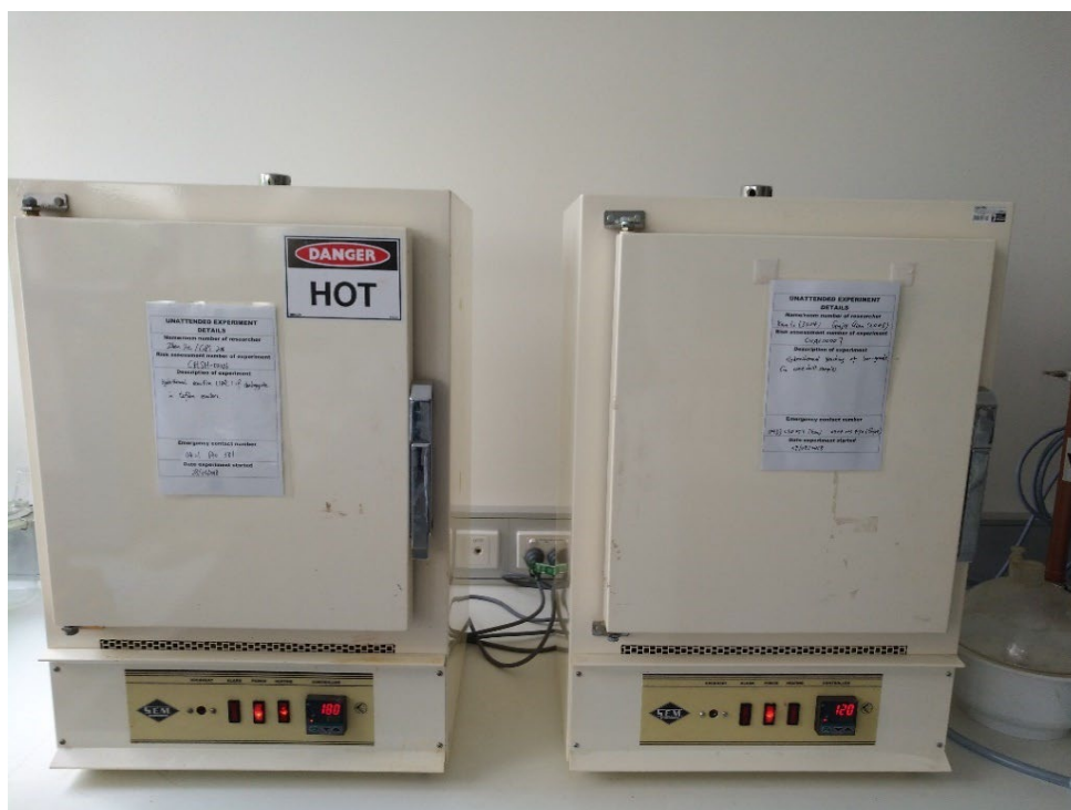
Figure 14 The ovens used in this research project to heat up. The maximum temperature of ovens is 500°C.
