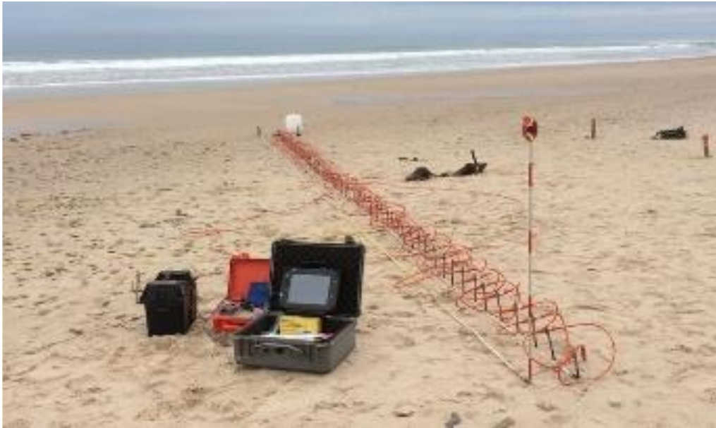
Figure 2. ERT survey equipment and linear probe array, Ida shipwreck site, Port Willunga Beach (photo by Kleanthis Simyrdanis).
